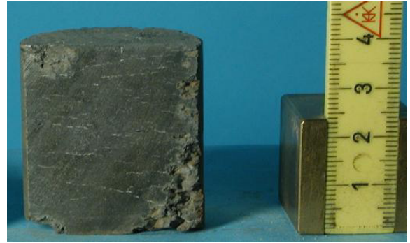
Figure 10: Sample of Draupen shale after CO 2 percolation
