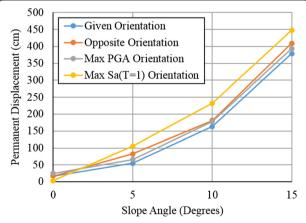
**Fig. 10** Comparison of the effect of ground motion orientation on the maximum calculated permanent displacement
