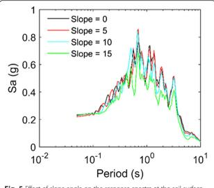
Fig. 5 Effect of slope angle on the response spectra at the soil surface
