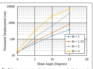
**Fig. 9** Maximum permanent displacement compared with slope angle and soil sensitivity
