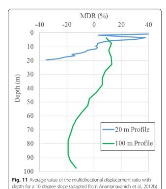
permanent displacements for the upper half of the profile than unidirectional shaking. At the surface, the 20 m and 100 m profiles predict about a 40 % and 20 % increase in permanent displacement for multidirectional shaking over unidirectional shaking, respectively.
