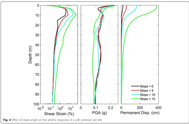
experiences a permanent displacement increases because the initial static shear strains increase.
