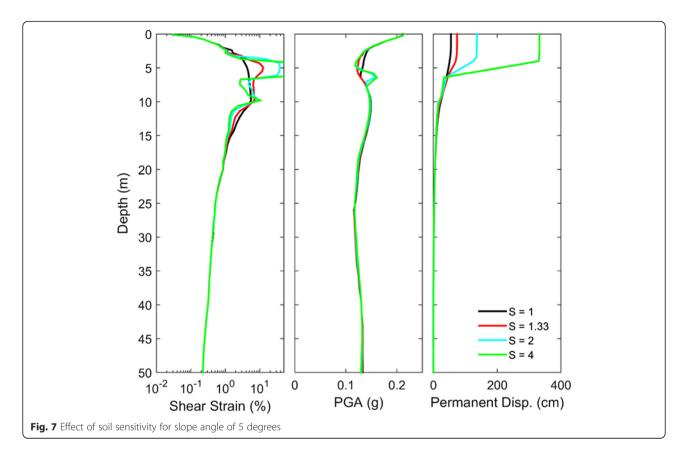
degrees, changing the soil sensitivity from 1 to 4 increases the maximum permanent displacement from 55 cm to 330 cm. For a soil with high sensitivity, the mobilized shear strength during the earthquake may fall below the shear stress that is required for static stability. When that happens, the slope essentially fails and the
