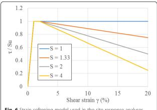
Fig. 6 Strain softening model used in the site response analyses
