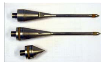
Figure 1. Piezoprobe and piezocone (DeGroot and Lunne 2002).
