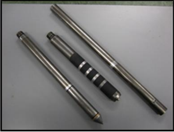
Figure 2 Example of R-CPTU probe (NIFS-report 2015-126).
