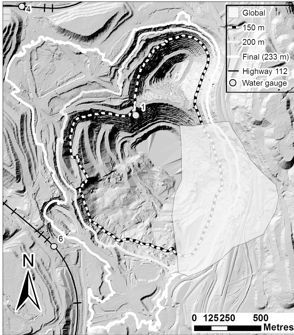
Fig. 2. Geometry of the Global rockslide scenario of 50 M m 3 . Three contour lines were added for elevations 150, 200 and 233 m.
