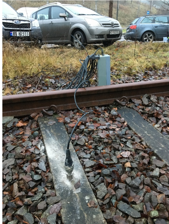
Figure 13: Simulated rock fall tests on an abandoned rail section. The geophones were mounted directly on the sleepers and a sledgehammer was used to generate shockwaves in the tracks.
