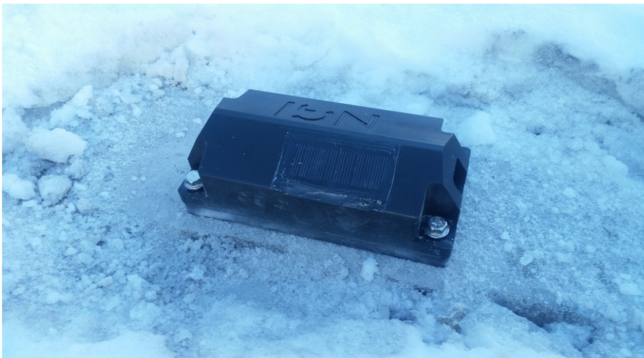
Figure 6: One of the sensor units installed on site. The enclosure encapsulates the sensors, data acquisition unit, radio module, antenna and battery. The only external components are the miniature solar panel visible on the lid, and a debug connector (not visible on the image). The sensor units are self-contained with no external cables.
