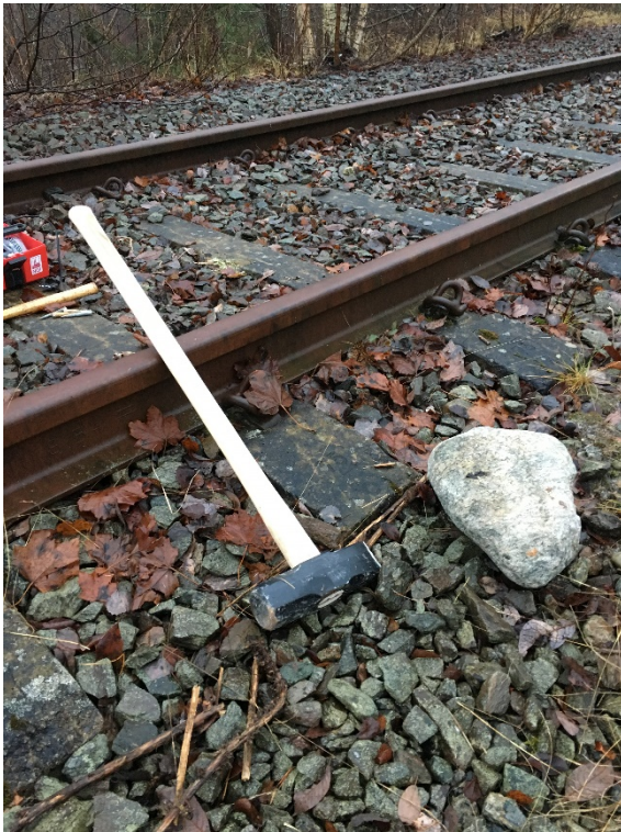
Figure 13: Simulated rock fall tests on an abandoned rail section. The geophones were mounted directly on the sleepers and a sledgehammer was used to generate shockwaves in the tracks.
