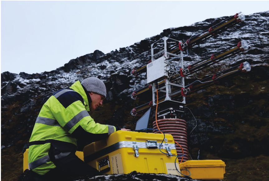
Figure 2.2. NGI engineers deploy the GAMMA Portable Radar Interferometer (GPRI) instrument to scan for line of sight deformation along a rock face.
