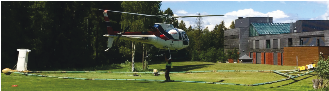
Figure 2.6. Airborne Electromagnetic Mapping (AEM) technique deployed by NGI engineers at a site in Horten.
