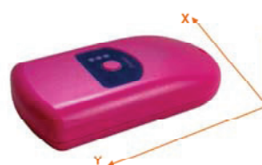
Figure 3: IMU (inertial measurement unit) unit that can sense accelerations, magnetic field of the Earth, and angular velocities. (48mm x 85mm x 15 mm)
