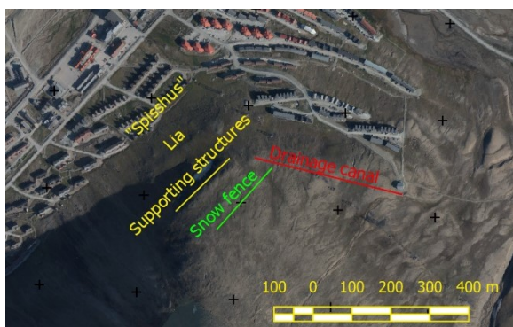
Figure 6. Schematic figure of location of mitigation measures. Aerial photo: Norwegian Polar Institute
