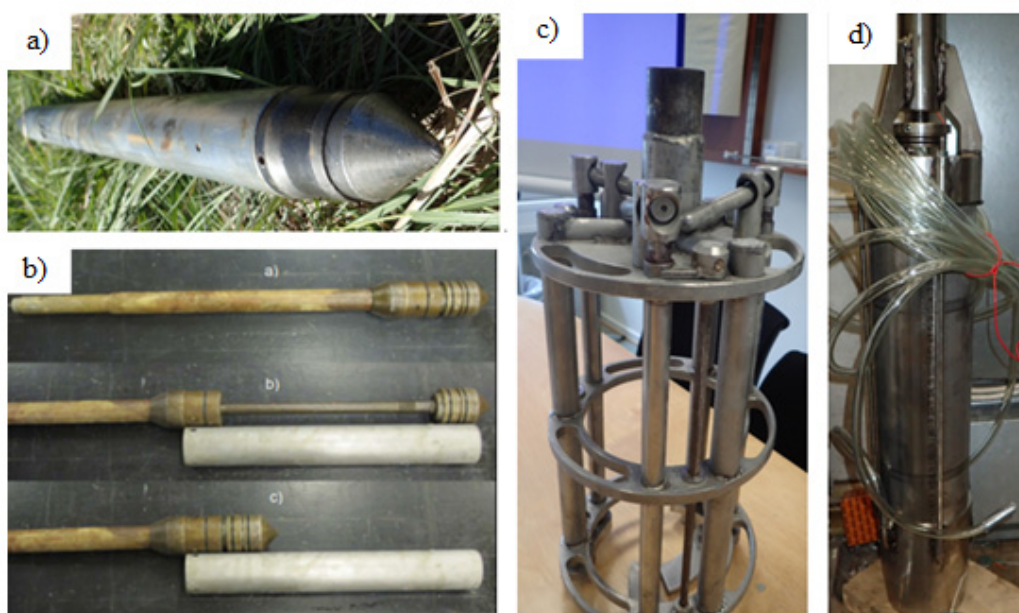
Figure 7. Samplers employed at Perniö site: a) ST:1 50 mm piston, b) Aalto 86 mm piston, c) Mini-block, d) TUT 132 tube.
