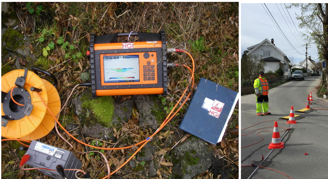
Figure 5.3. Basic principle of electrical resistivity imaging (top). It is possible to determine earth resistivity \rho by driving a current I into the ground and measuring the resulting potentials \Delta V (Figure from Knödel et al., 2007). Electric resistivity tomography (ERT) with field instrument linked to electrodes planted in the ground using electrical cables (lower).
