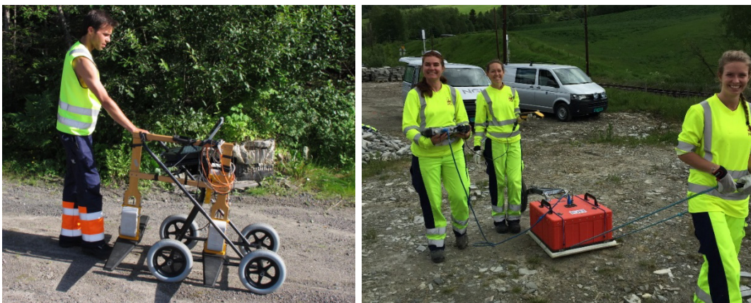
Figure 5.5 GPR technology: the instrument can be easily rolled over even ground.
