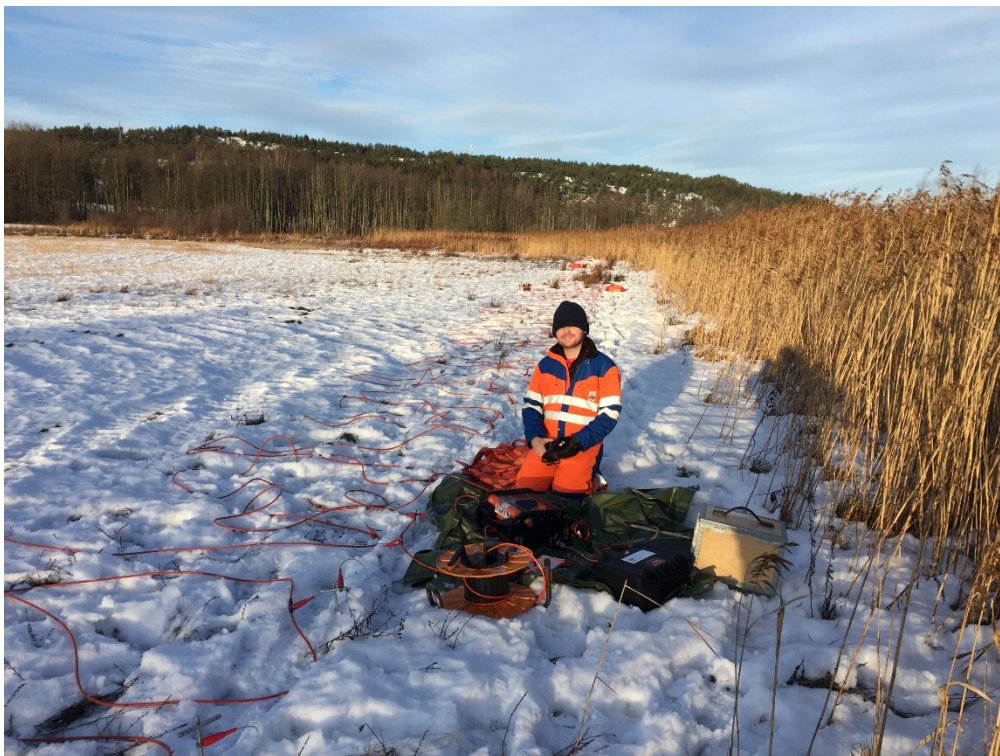
Figure A4 ERT acquisition along profile L1 at Onsøy old test site.
