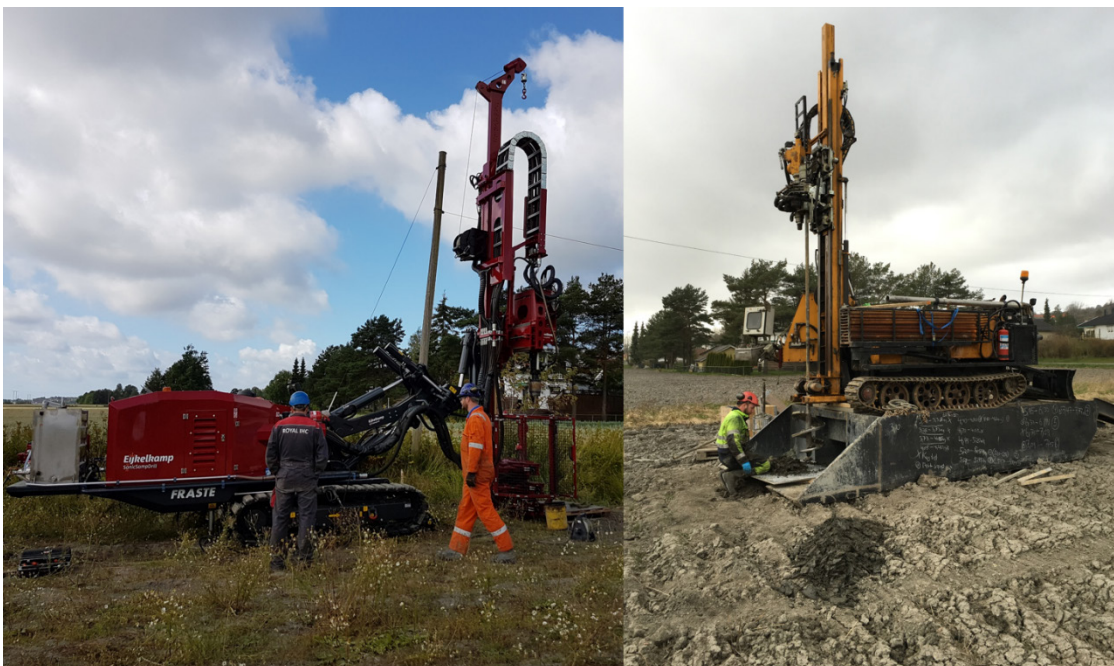
Figure 4.15.1 Left hand side: 76 mm sampling rig. Right hand side: block sampling setup
