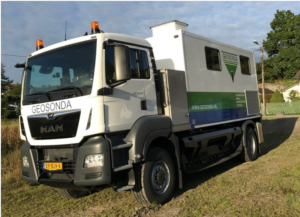
Figure 4.7.1 Geomil rig used for cone penetration testing
