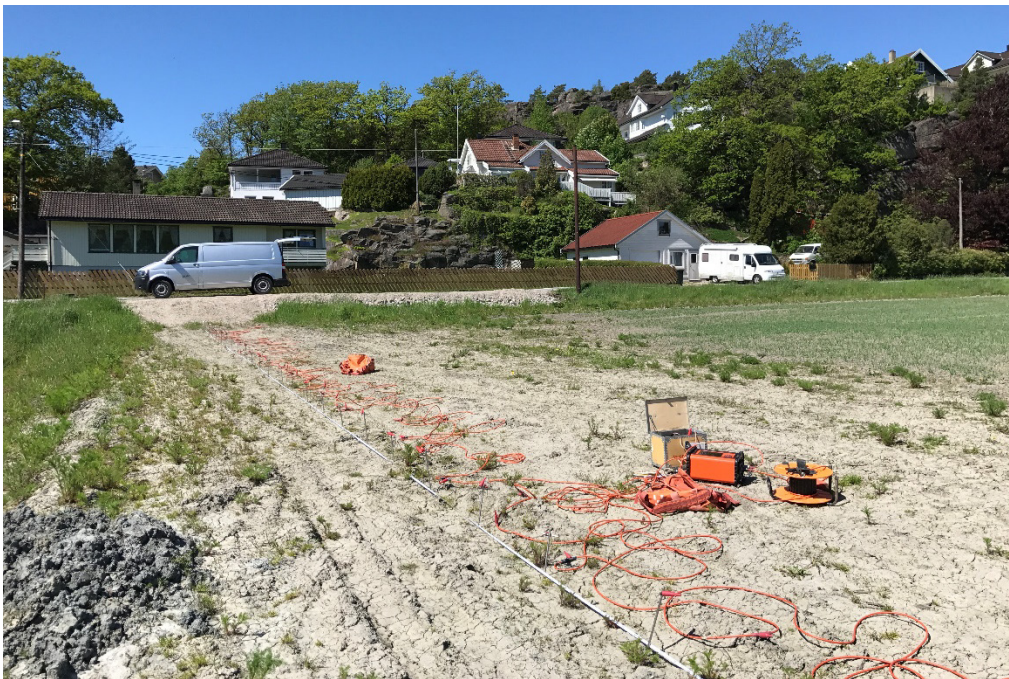
Figure A7 ERT acquisition along profile L4 at Onsøy new test site in April 2017.
