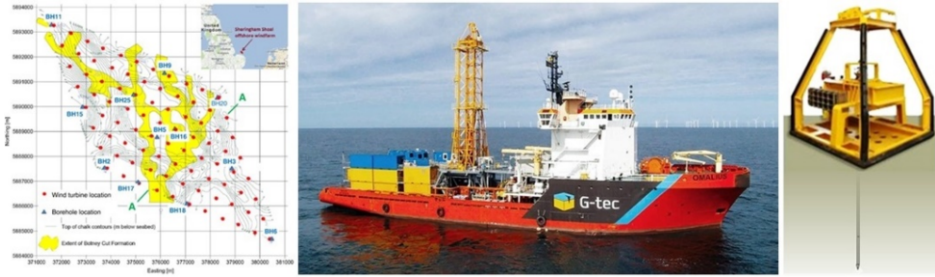
Figure 10. Left to right: Borehole and wind turbine location plan [5], geotechnical drilling vessel and seabed CPT rig.
