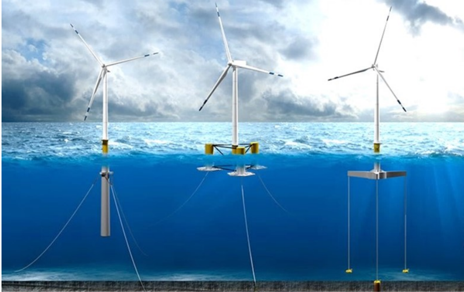
Figure 23. From left to right: SPAR, Semisub and TLP type of OWT floaters (Illustration: DNV-GL).
