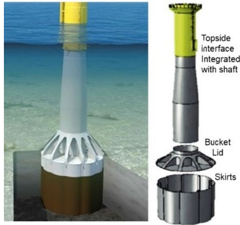
Figure 19. Mono bucket foundation (illustration: Universal foundations).
