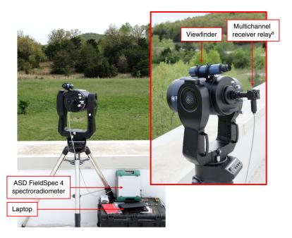
**Fig. 4** Labeled photograph of the field setup as used to collect intermediate-range spectral reflectance measurements with the SOLAS telescope-enhanced receiver.
