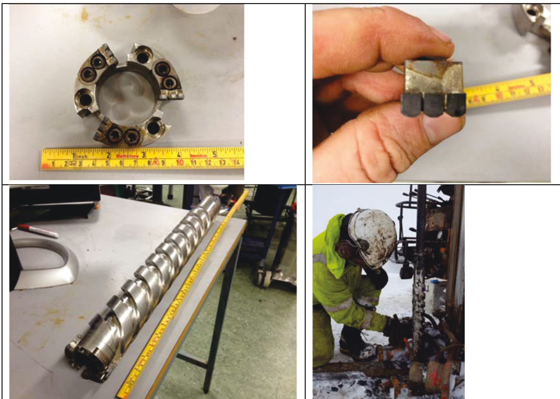
Figure 5 The SINTEF permafrost corer; drill piece (top left), PCD inserts (top right), frost corer assembled (lower left) and sampling in Adventdalen (bottom right).
