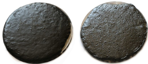
(e) Sandy asphalt mastic, left, KFS; right, ZFS
