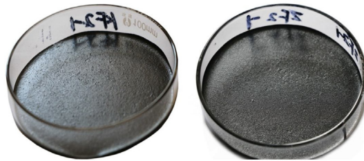
(c) Asphalt mastic (bitumen: filler = 1:2), left, KF2-1; right, ZF2-1
