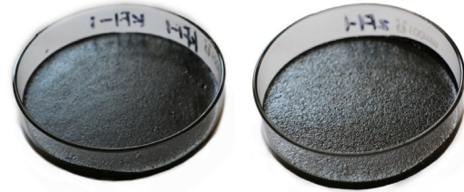
(b) Asphalt mastic (bitumen: filler = 1:1), left, KF1-1; right, ZF1-1
