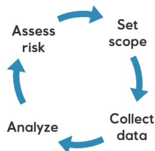
Figure 2-1 In a risk-based GCS monitoring strategy, an initial monitoring scope is based on available information, and adjusted continuously as new information becomes available. Adjustment of the monitoring scope may be in terms of frequency of surveys, focus on target areas, and choice of sensor technologies. As confidence in the storage site is built, the monitoring scope may be down-scaled.
