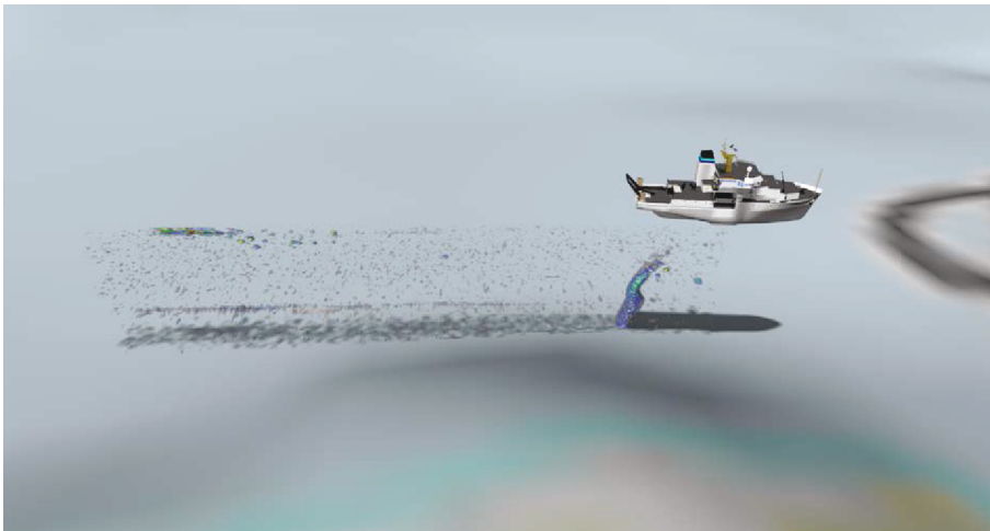
Figure 3-3 EM712 MBES image acquired during the ACT4storage project. CO 2 bubbles were released at a rate of 1.3 l/min at the seabed and can be recognized as a "flare" shaped structure rising ~40 m above the release point at the seabed.
