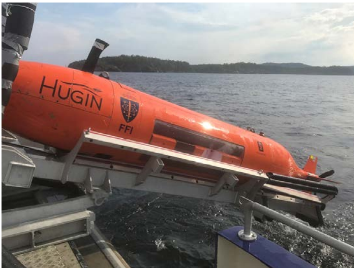
Figure 3-7 The HISAS mounted on the HUGIN AUV, with capabilities for mapping the seabed and detecting gas seeps in the water column. This image was taken in Horten during the ACT4storage nearshore experiment.
