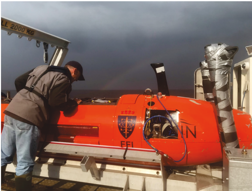
Figure 8-1 HUGIN operator checking that the chemical sensors are ready for deployment. The chemical sensors are integrated on the top, and the starboard side of the HISAS 1030 sonar is partially visible in dark red.
