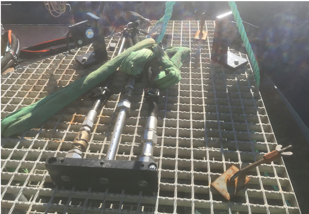
Figure 4-6 Three hoses were used to facilitate release of seawater with elevated CO 2 levels, and CO 2 or air in gas form (bubbles) with different orifice sizes and spatial distribution. The hose to the left was used for seawater, with a single 10 mm hole as release point. The middle and rightmost hoses were used for air and CO 2 in gas phase. The middle hose has 8 3-mm holes, and the rightmost hose has a single 5 mm hole. The orifice size was used to control the bubble size distribution. A video camera and external light source was used to document and verify the leak.
