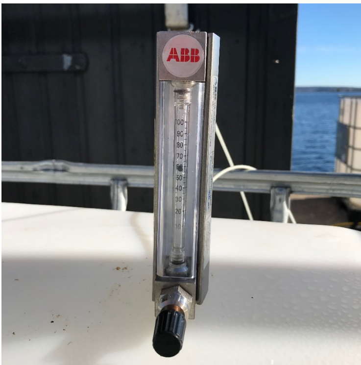
Figure 4-8 Flow meter used to accurately determine the flow rate of CO 2 in gas phase. Here, the black sphere is at 60 %, which corresponds to a leak rate of 0.75 l/min (100% corresponds to 1 l/min).
