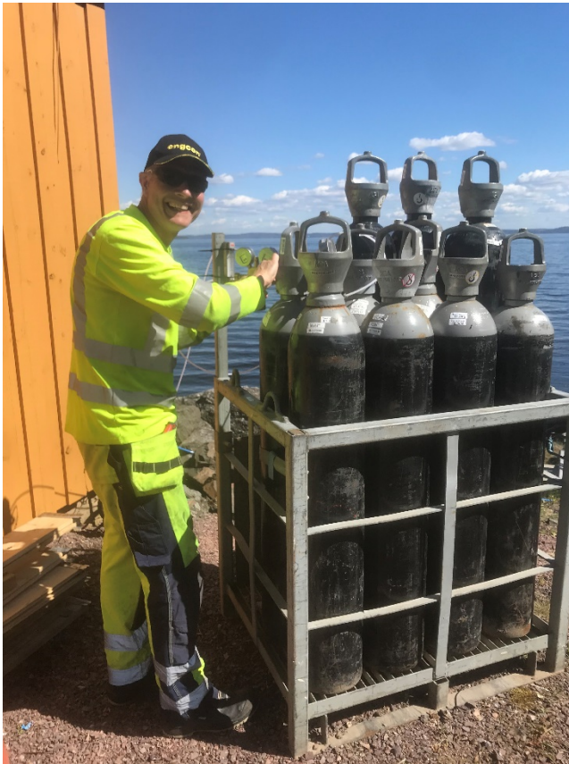
Figure 4-4 CO 2 containers used during the controlled release experiments. CO 2 was either released directly in gas phase (via flow meters to control and document the flow) or dissolved in seawater to mimic CO 2 -enriched fluids entering the water column.
