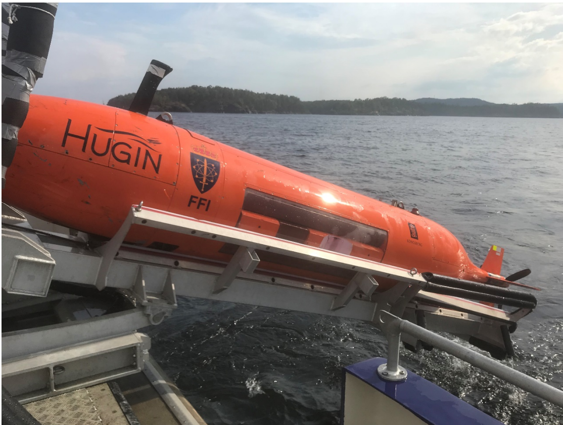
Figure 5-5 HUGIN AUV during deployment from the vessel Sølvkrona. The sensor payload was updated to suit this experiment, including CONTROS HydroC CO 2 and CONTROS HydroFlash O 2 , CONTROS HydroC CH 4 , Franatech CO 2 , Franatech CH 4 , Idronaut pH, and HISAS synthetic aperture sonar.
