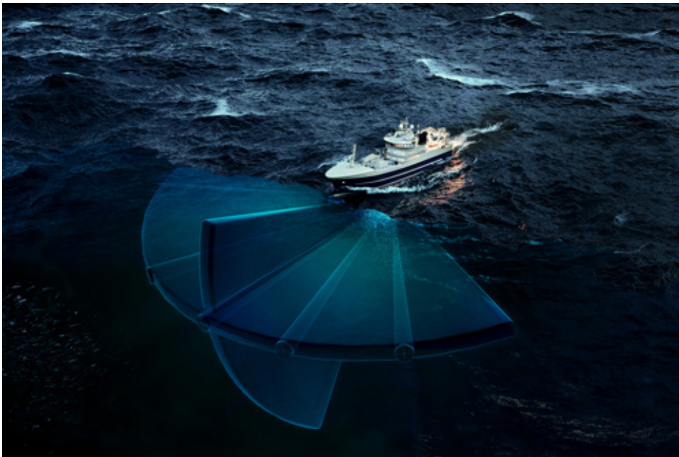
Figure 10-14 Illustration of the swath coverage offered by the SN90 in both the along-track and across-track directions. The beamwidths and beam angles can be tuned to suit operational needs. Image courtesy: Simrad.com
