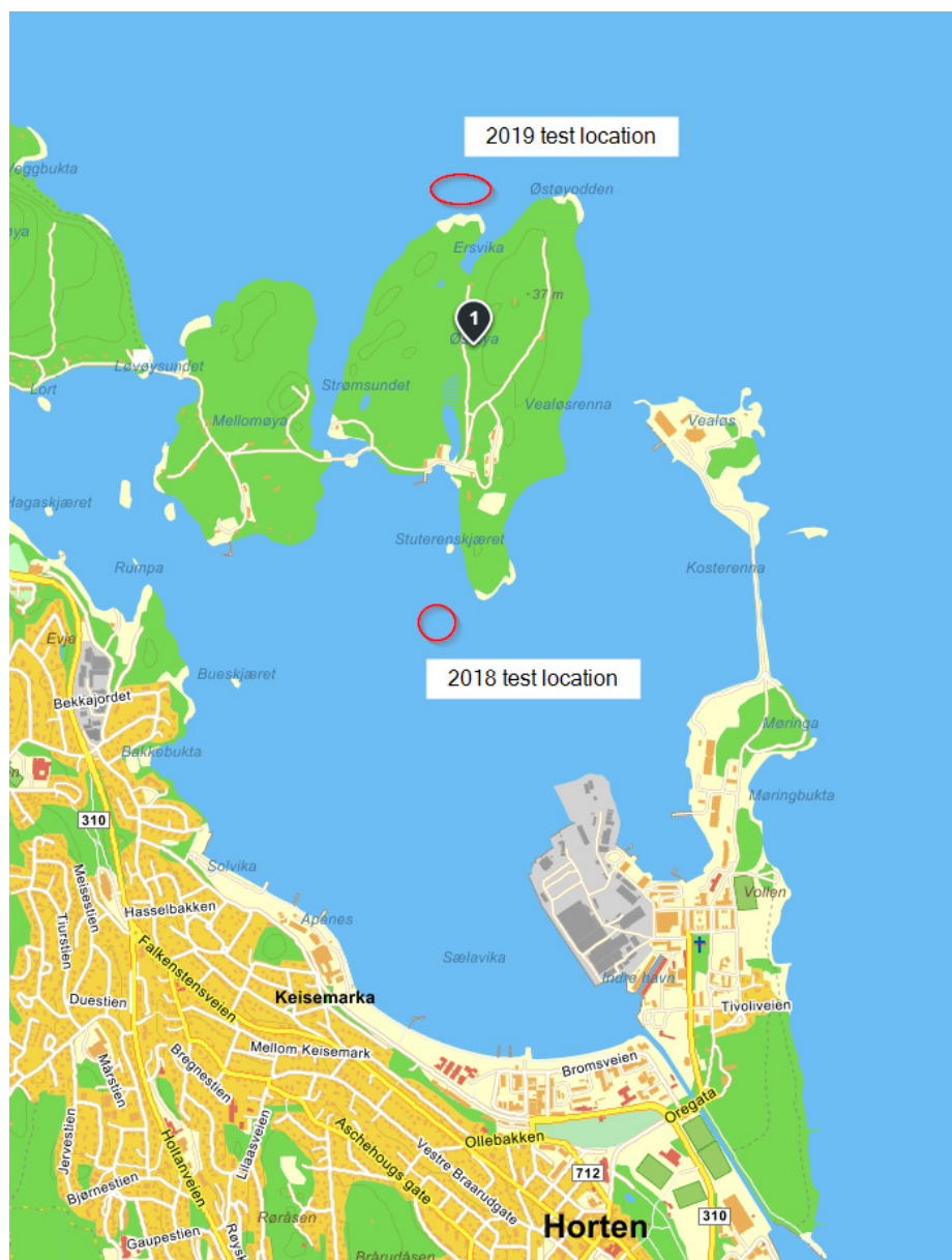
Figure 3-1 Test locations for the 2018 and 2019 nearshore tests, respectively. The 2018 tests were carried out in a protected environment with 16-18 m water depth and anoxic conditions. The 2019 tests were moved to more representative conditions with oxic conditions and 60 m water depth.
