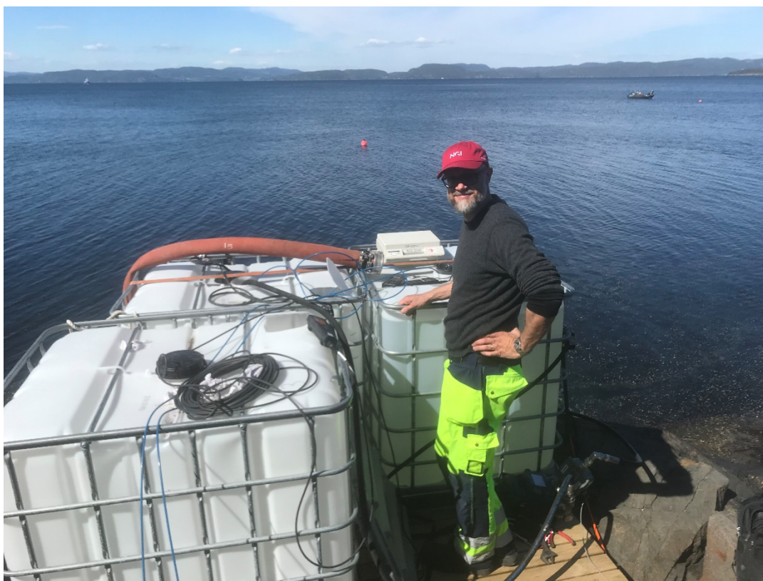
Figure 4-5 CO 2 -enriched pore fluids were simulated by adding appropriate amounts of CO 2 into seawater in three 1000-litre tanks. The contents were then released in a controlled way using a pump and a hose placed at the seabed. The release point is located 100 m from shore, to the left of the red buoy. AlSeamar's SeaExplorer glider was deployed from the small boat in the upper right corner of this image.
