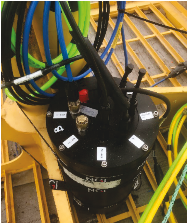
Figure 5-4 Subsea container designed and built at NGI, supplying sensors with adequate power and ensuring data communication
