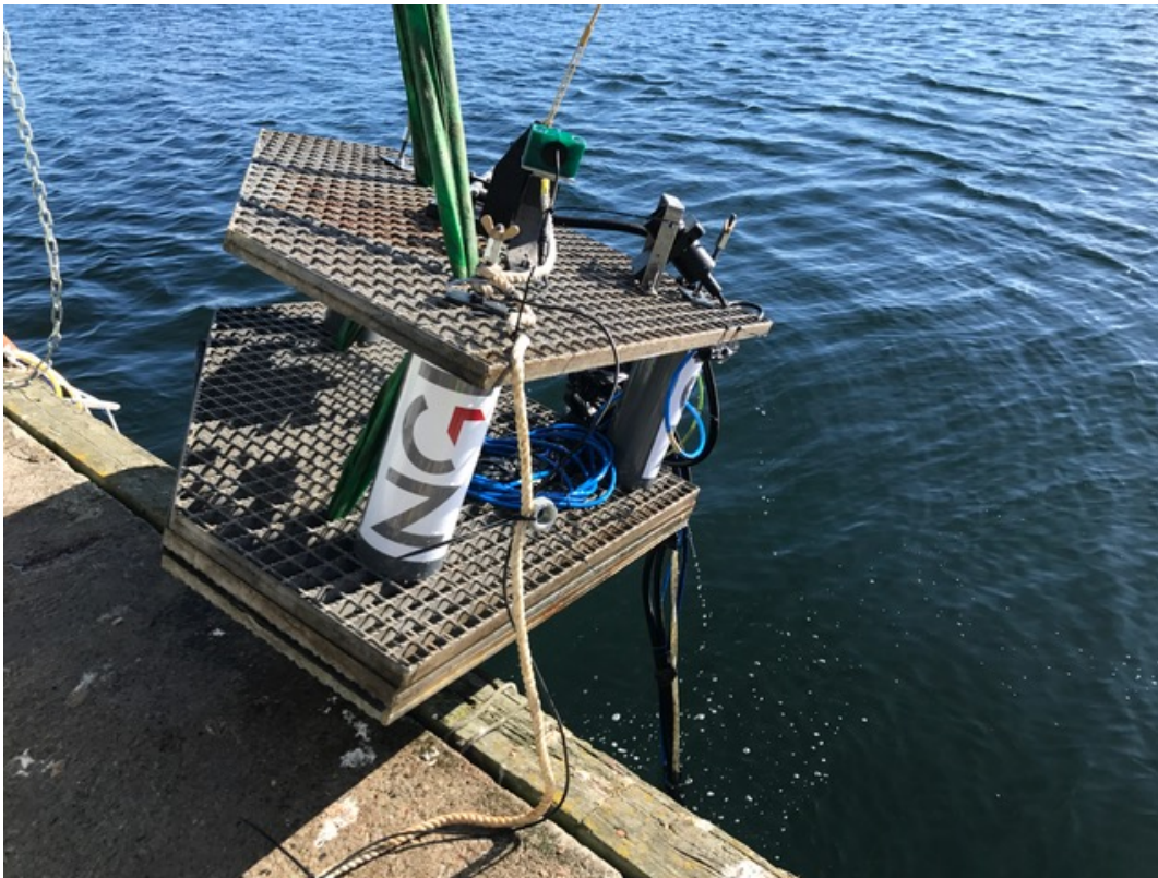
Figure 4-1 Leak frame developed by NGI for controlled release of air, CO 2 bubbles, and seawater saturated with CO 2 . The fluid- and gas flow was controlled and documented from shore, and a subsea video camera was placed on the frame to verify the simulated leak.
