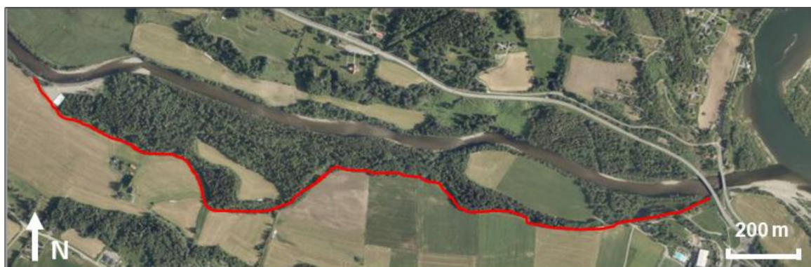
Figure 4. The lower reaches of the river Gausa, where it enters the main river Gudbrandsdalslågen (far right). The proposed receded flood barrier (Location G1 in Figure 3) is marked with red. The original flood barrier follows the southern riverbank.
