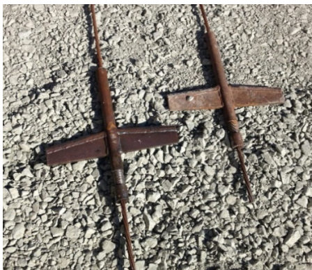
Figure 4. Photograph of the RCP probes to be installed in the lime-cement columns
