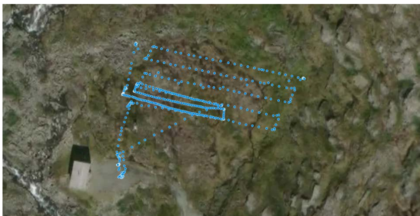
Figure 4-7. UAS flight lines and image locations placed in Google Maps using Pix4D.
