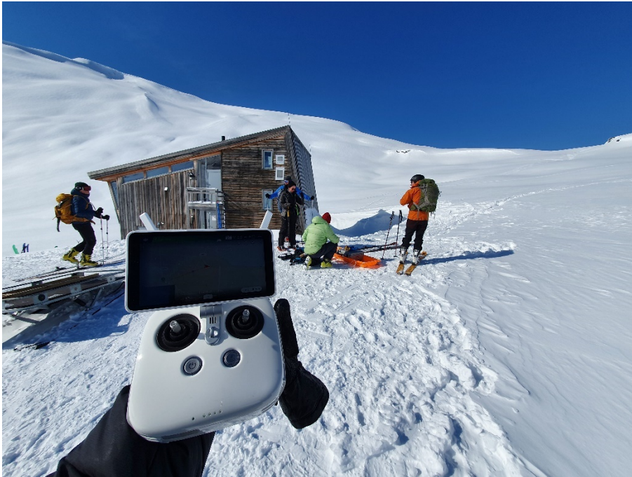
Figure 5-2. DJI flight controller used for planning and executing flight missions in the field. (Photo: Sean Salazar)
