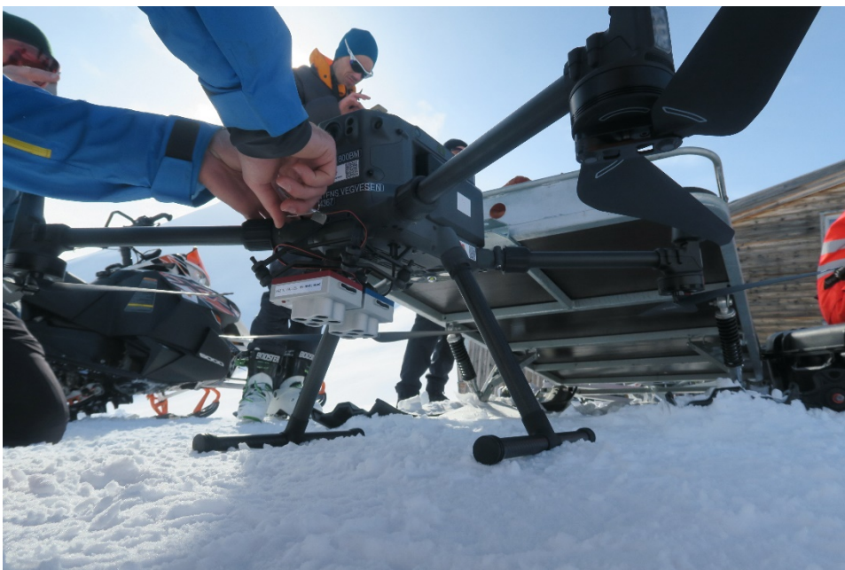
Figure 4-1. The MicaSense multispectral camera mounted on NPRA’s DJI Matrice 300 RTK aircraft. An external GNSS receiver was also mounted on the UAS for geotagging multispectral data. The camera was controlled directly from the ground via a WiFi interface. (Photo: Tore Humstad)
