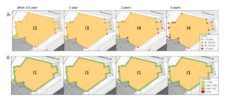
Figure 9. Classification of the groundwork impact according to Rankin 1998 (see Table 1). Top row: vertical settlements of the corner points. Bottom row: rotation (or slope) of the building walls.
