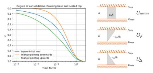
Figure 5. Triangular isochrone and corresponding U-T curve (from Terzaghi & Frohlich 1936)
