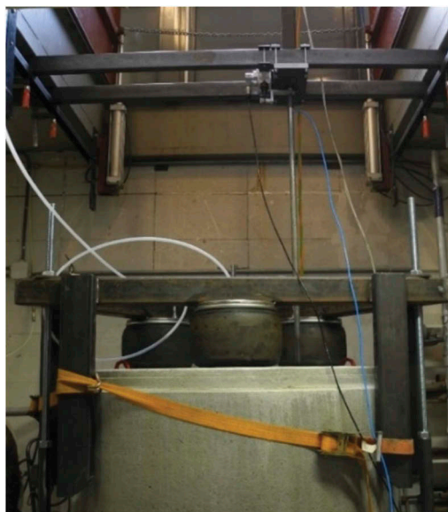
Figure 3. The overburden loading framework on the chamber. Above: the actuator and the probe fixed to a framework.
