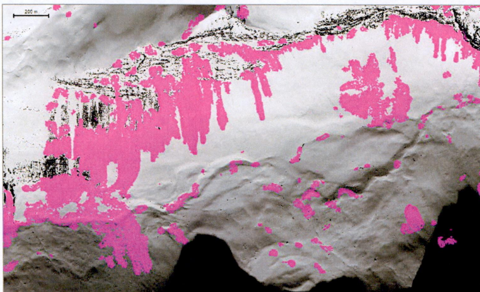
Figure 1: Identification of snow avalanches in a WorldView-1 image using an algorithm developed for Leica ADS-40 imagery.
