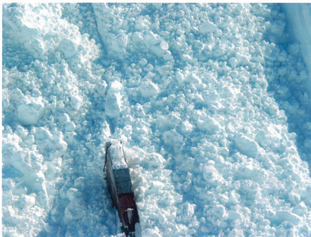
Figure 2.22: Avalanche 20050416 15:00: Sensor status after the event; the width of concrete wedge is about 0.6 m. (Photo by Krister Kristensen)
