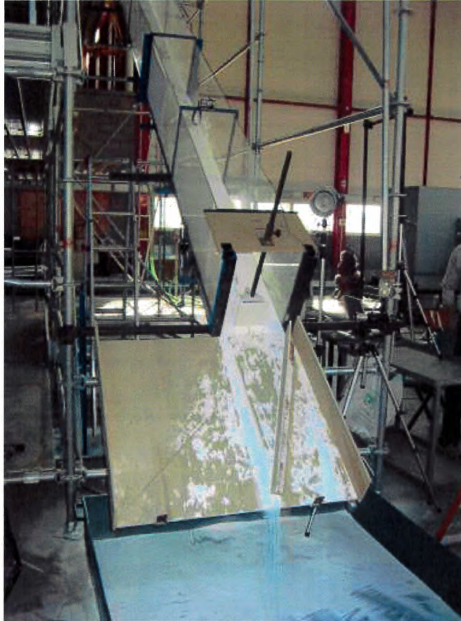
Figure 2: The 7.5 m long experimental chute with an attached plywood plate for the mounting of deflecting dams. A wedge with a 60^\circ top angle and a deflecting dam with a 20^\circ deflecting angle are mounted on the chute. The masts were mounted about 20 cm above the lower end of the chute.
