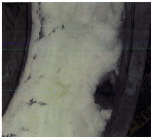
Figure 3.2: First tests with snow: shear bands appear near the inner cylinder.
