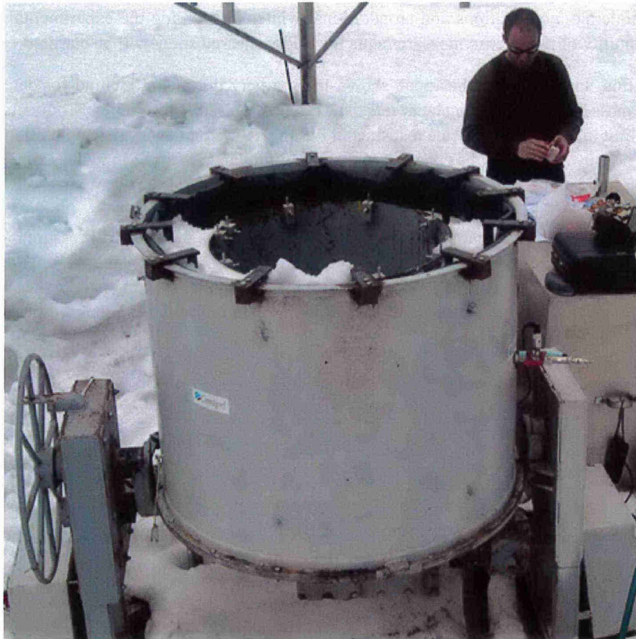
Figure 3.1: The annular snow rheometer during the tests at Col du Lac Blanc, winter 2005/2006. The snow to be tested is filled into the annular space between the two concentric drums. The inflatable black membrane lining the outer drum is clearly visible.
