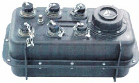
Figure 1.7.1: 6-channel Reftek seismic recorder acquired for installation in Ryggfonn.
