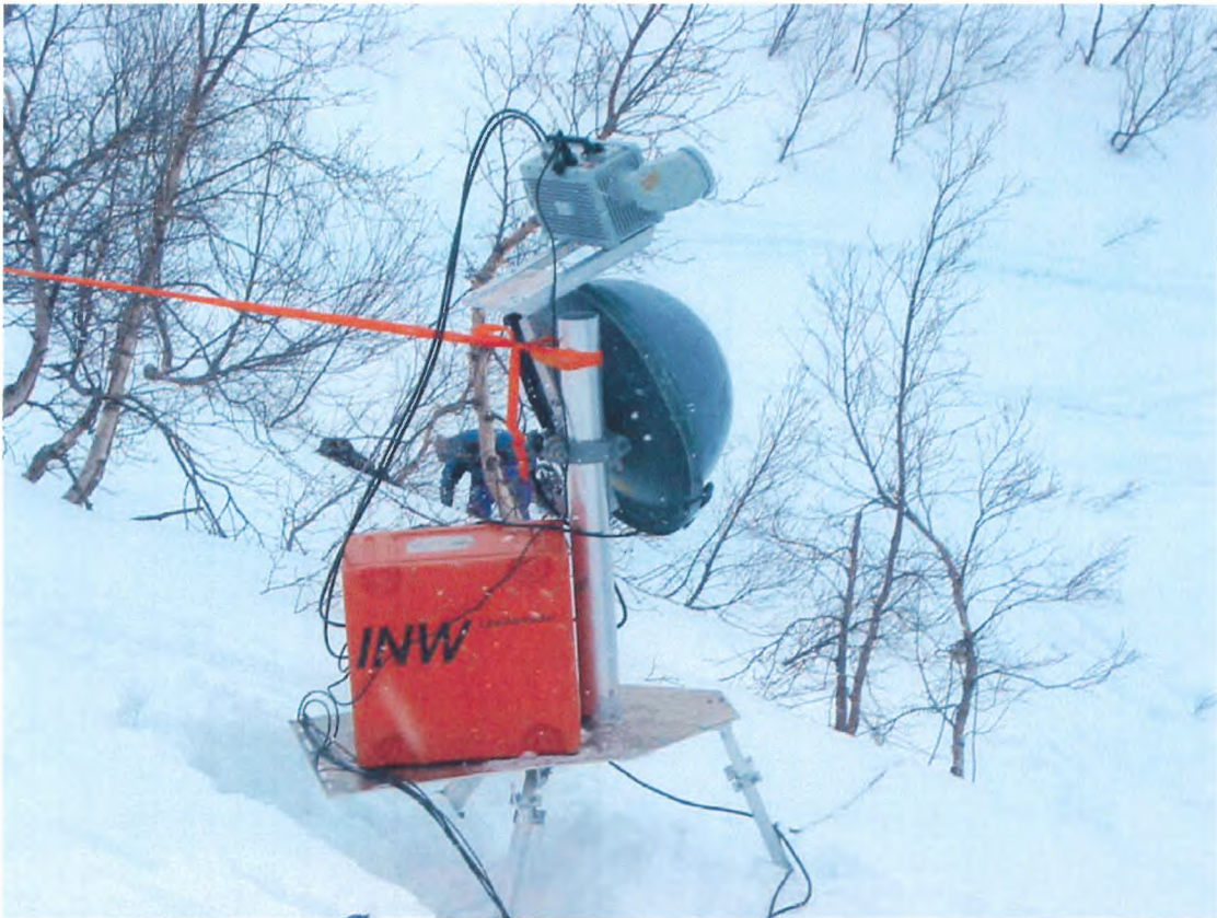
Figure 3.1.8 Antenna of the AIATR radar facing the avalanche path
