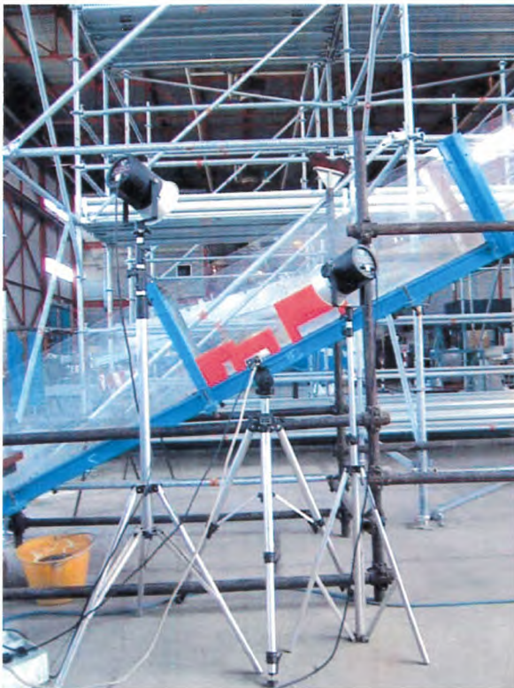
Figure 2 - Side view of the chute, with indication of the recording area
