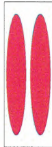
Figure 9. One-dimensional array of two sensors designed to reduce bias from vertical velocities. The active region of the sensors averages over a large vertical region to reduce bias.
