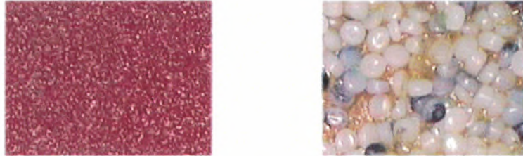
Figure 3 - Sand paper bed (left) and glued particles bed (right)
