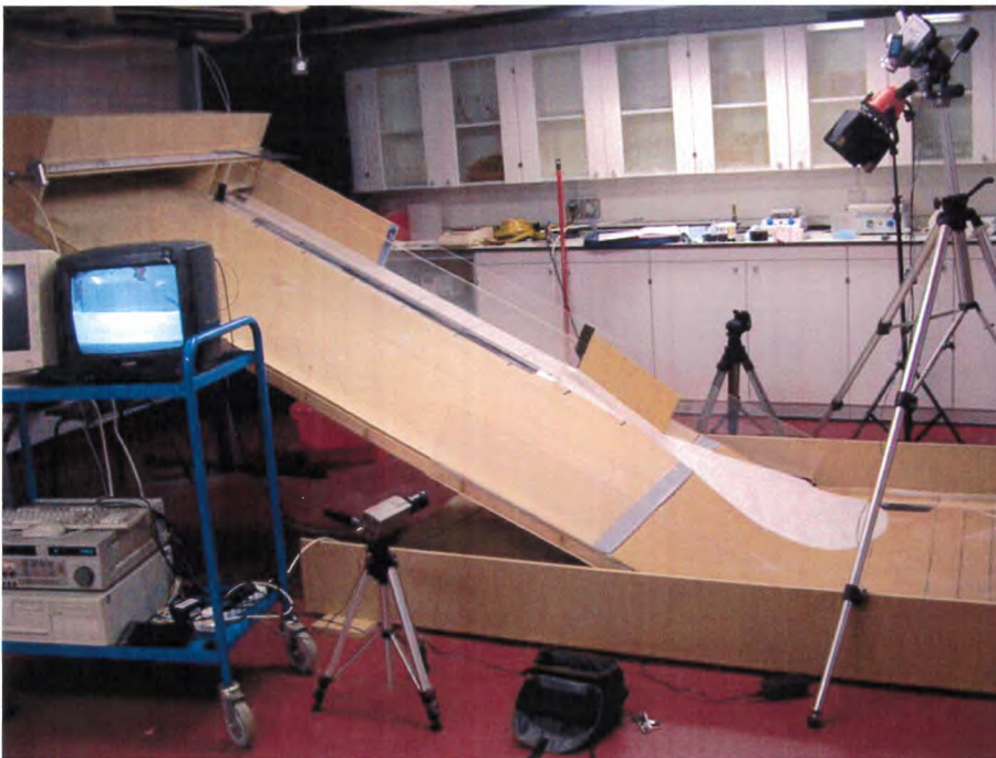
Figure 3.4.11 A photograph of the experimental set-up of the wooden chute at Bristol University.
