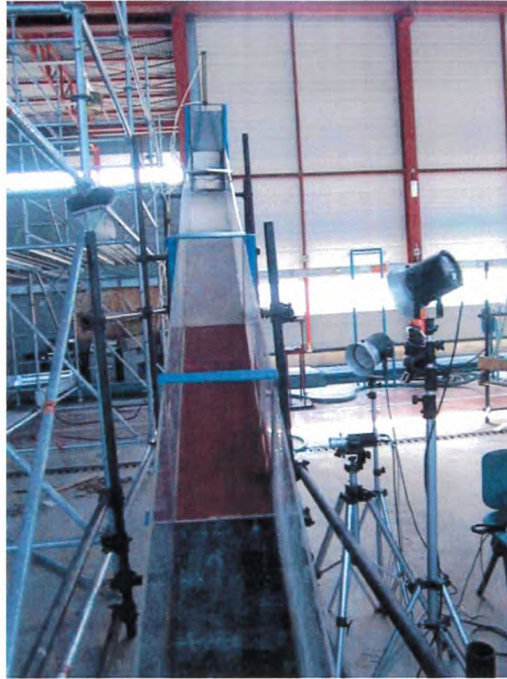
Figure 15 - View of the chute covered with sand paper in the area of the recording section (up to about 1 meter upstream)
