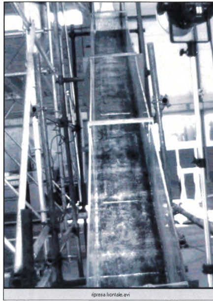
Figure 5 - Front view of the chute; the white marks on the bed are used to measure front position versus time, i.e. front celerity
