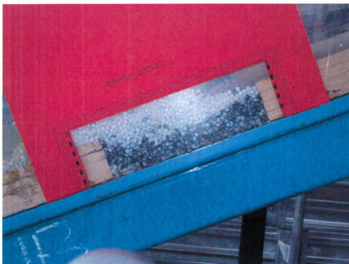
Figure 4.2.6. An image showing an erosion experiment in the Pavia chutes. The white flowing grains have entrained the darker underlying substrate, the surface of which was originally flush with the adjacent chute bed.
