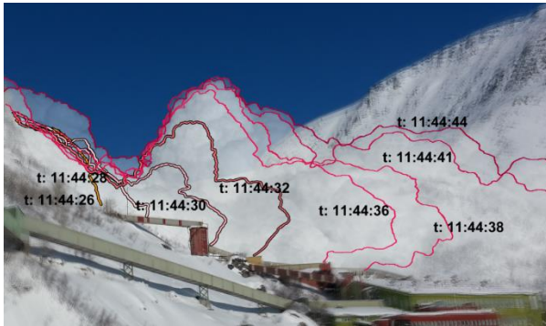
Fig. 7: Outlines (superimposed on photograph of time step 11:44:26) of the lateral front of the powder cloud during a 18 second time interval. The time presented on the photograph is the camera time. The accuracy of the camera time measurement is unknown.
