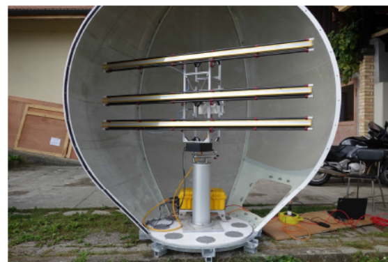
Fig. 2: Gamma Portable Radar Interferometer (GPRI) with a height of about 2.2 m and a weight of 45 kg, installed in a radome at SLF.
