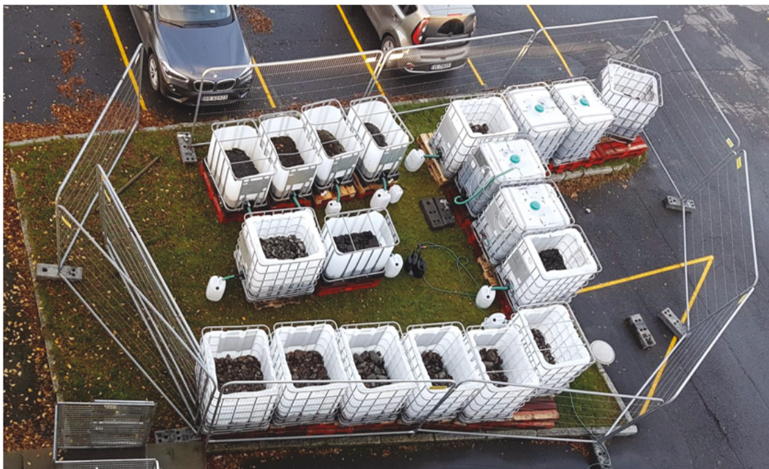
Figure 6 Overview of containers for leaching experiments. Five containers "inherited" from the Norwegian Public Road Authorities are also in the photo.
