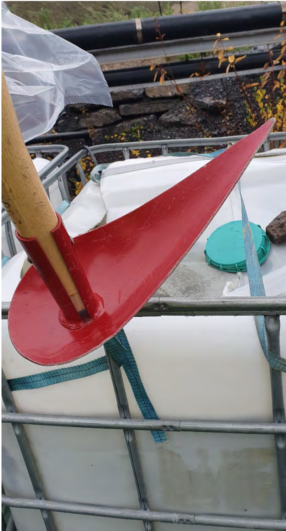
Figure 18 Sampling of rock from the DF and DS containers was done with this, but it was not very well suited. The metal part was a bit too long, and to collect a sample, the whole shaft and the holding hand had to be submerged. For the next sampling, use something with shorter tip or longer handle.
