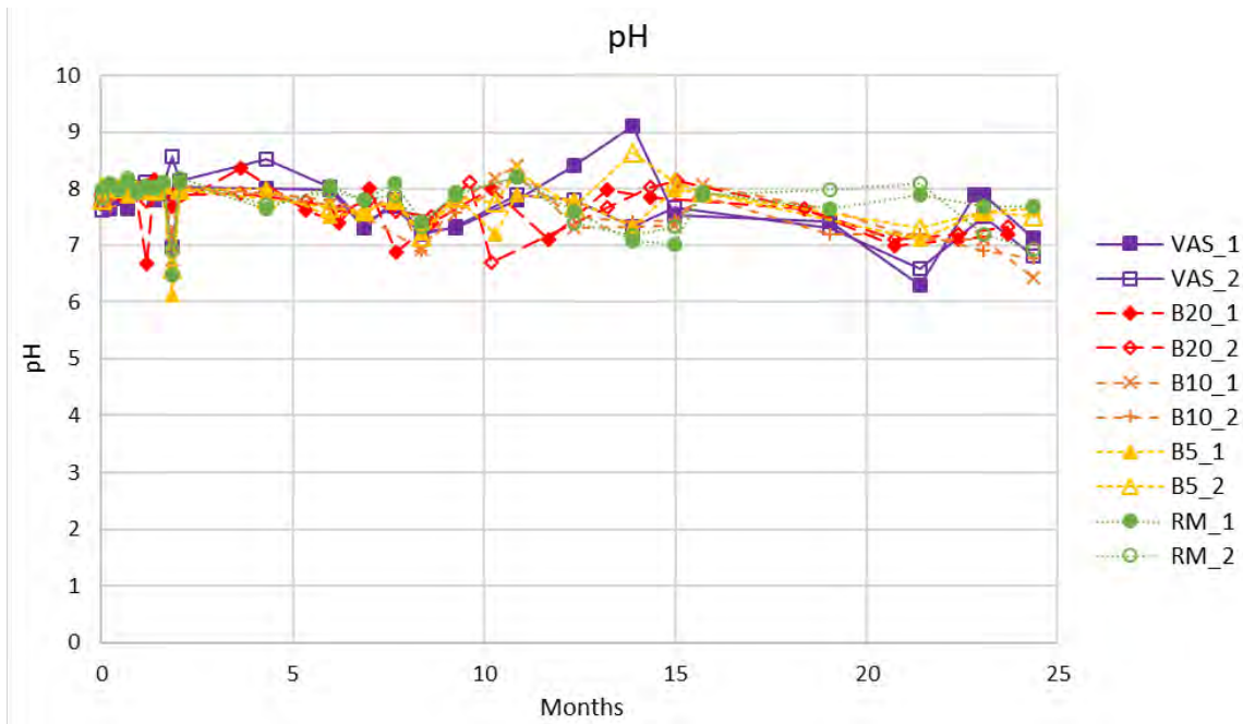
Figure 20 pH values measured with time for the first 24 months of the containers experiments with alum shale from Kleggerud mixed with rhomb porphyry. VAS = pure alum shale, RM = rhomb porphyry, B20 has 20 % alum shale and so on.
