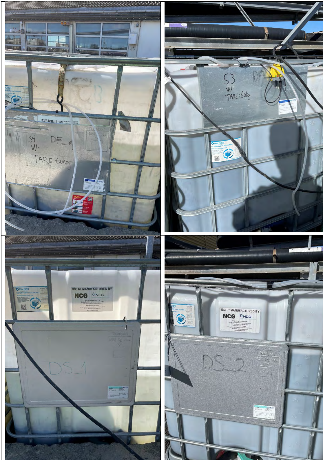
Figure 8 Water levels in containers (from top left) DF_1 (710 L), DF_2 (790 L), DS_1 (580 L) and DS_2 (800 L) some time after refill to 800 L after transport from Ullevål to Langøya. Photo: Kristofer Larsen, NOAH AS, ca. 11.04.2022.
