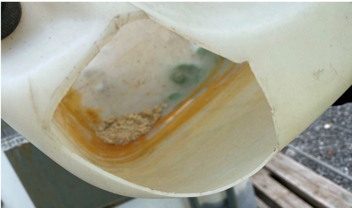
Figure 11 Precipitations observed in can collecting leachate from container G2 on 22.09.2022. It is unknown if this is new precipitate or leftover from the winter. Earlier, such precipitates have been observed after freezing periods.
