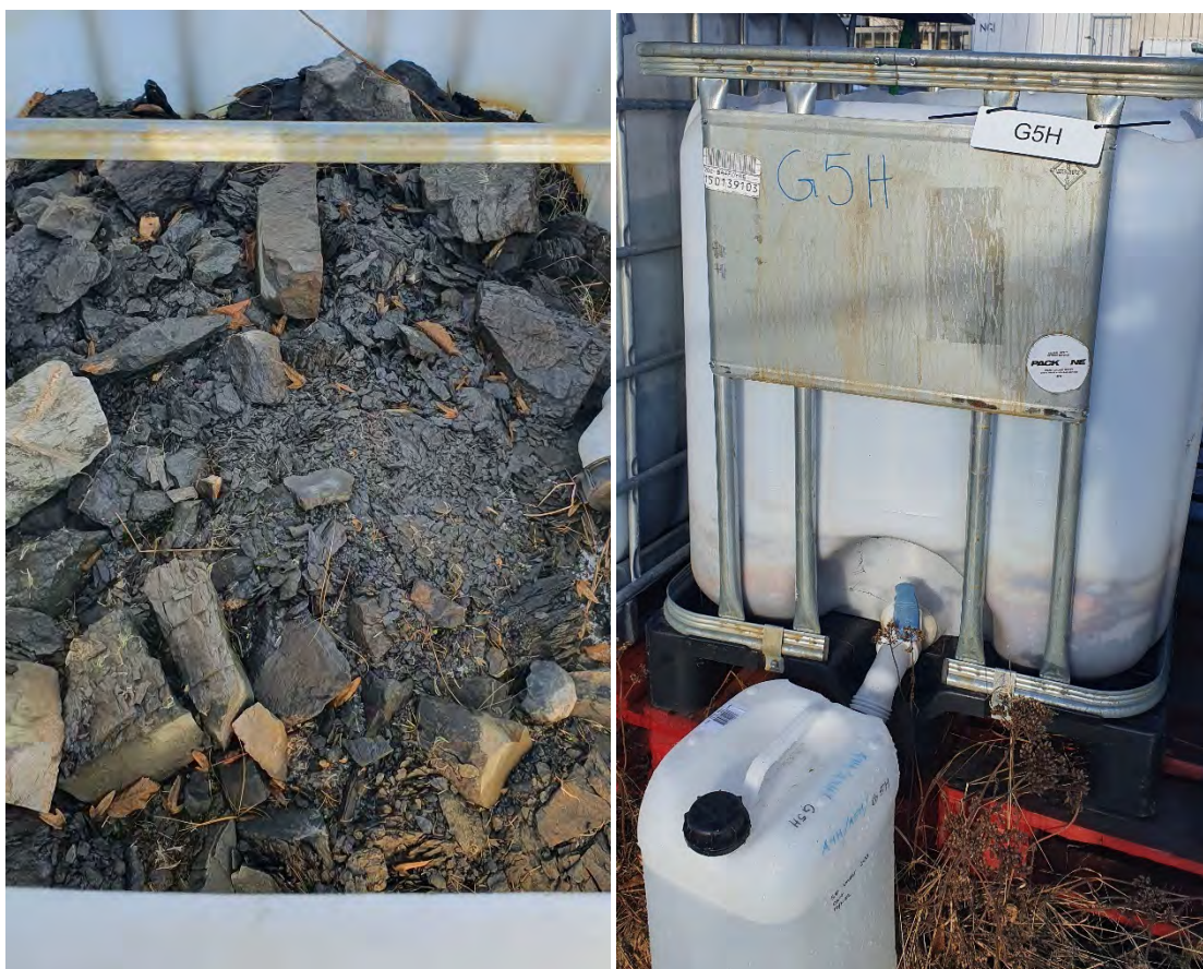
Figure 4 Pictures of unknown container (G5H/A4H/A5H) taken 24.02.2022. On the left, the disintegration of black shale can be seen. On the right, iron precipitates on the side of the container.
