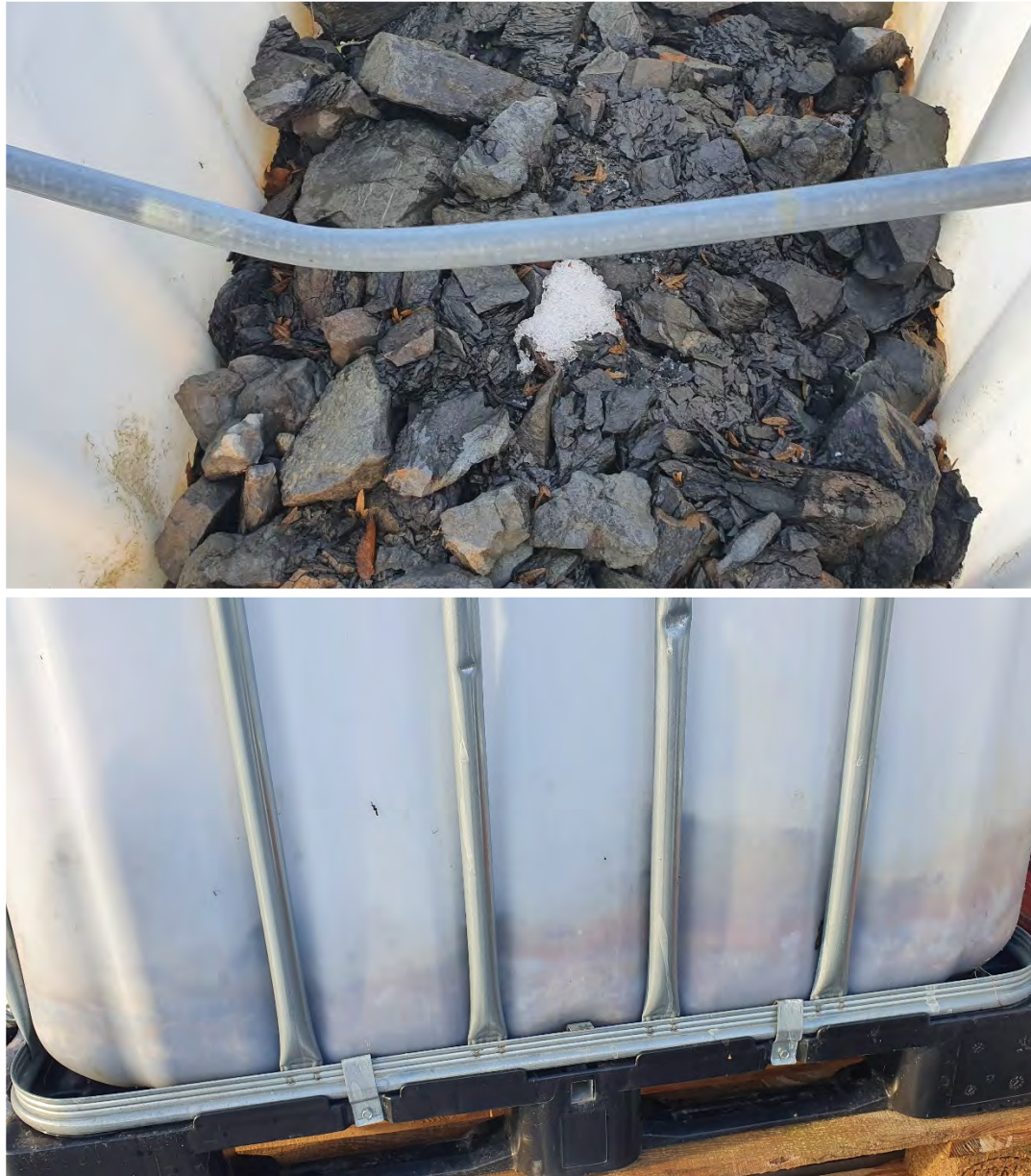
Figure 3 Pictures of container G4H taken 24.02.2022. Top: the disintegration of black shale can be seen. Bottom: iron precipitates on the side of the container.
