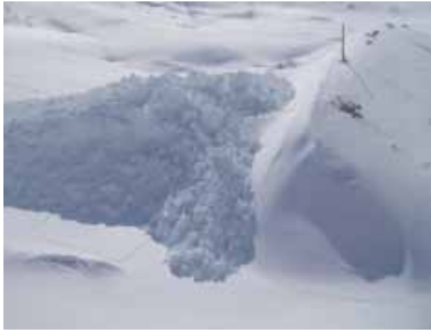
Figure 8.2: A wet-snow avalanche in front of the Ryggfonn catching dam that has piled up to a considerable height and also shows some tendency to divert sideways (photo: NGI).
