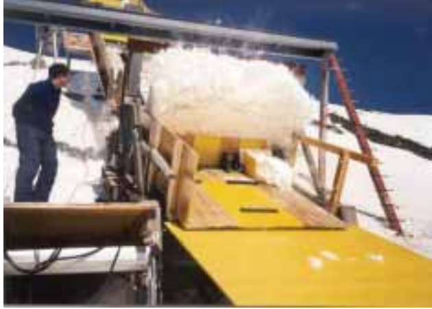
Figure 9.3: A photograph of the snow hitting a 60 cm high catching dam in the 34 m long chute at Weissfluhjoch (Hákonardóttir and others, 2003d). A part of the dam broke during this experiment as seen on the photograph.
