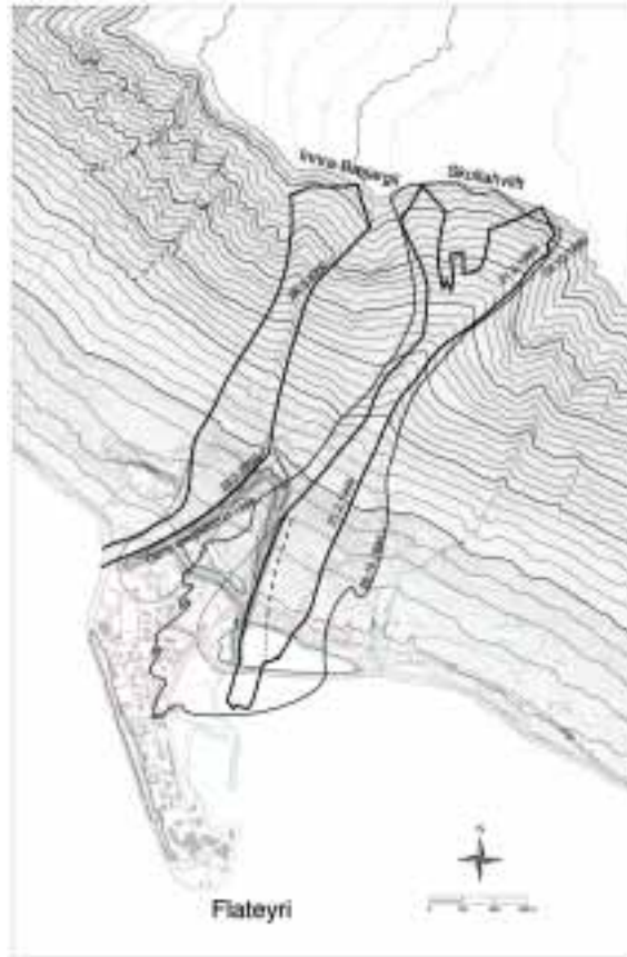
Figure 6.5: Outlines of avalanches that were deflected by the deflecting dams at Flateyri, northwestern Iceland, in 1999 and 2000. The outline of the catastrophic avalanche in 1995 is also shown. The channelised flow of the 1999 avalanche from Skollavilft along the deflecting dam is indicated by a dashed curve. Hypothetical outlines of the avalanches in 1999 and 2000 in the absence of the deflecting dams are shown as dotted curves. Due to the channelised flow along the dam, the run-out of the 1999 avalanche may have been increased by a distance on the order of 100 m.
