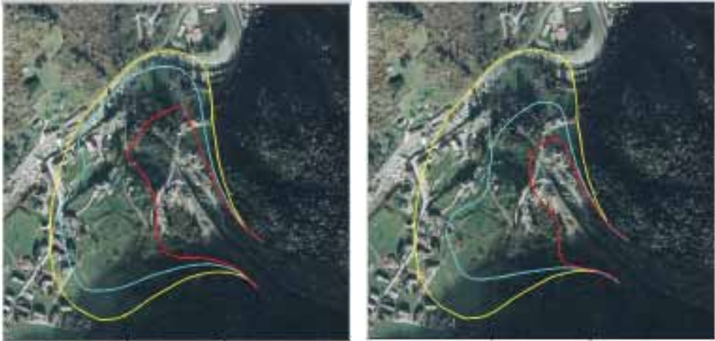
Figure G2: An example of the modification of an Italian hazard map after the construction of protective measures: The hazard map before the protective measure were built (left) and an updated map after the construction of protective measures (right) (both snow bridges in the release zone and a deflecting dam in the run-out zone). According to current Italian guidelines, the boundary of the yellow zone has remained unchanged. “Trabuchello” avalanche path, Isola di Fondra community, Brembana Valley, Italy, Central Alps.
