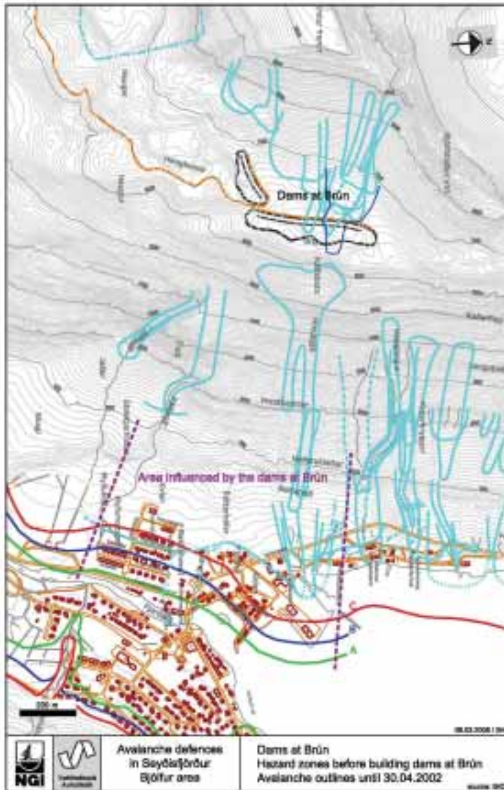
Figure C4: Dams at Seyðisfjörður, eastern Iceland (black curves). The map also shows the outlines of avalanches recorded before the construction of the dams (light blue curves, one highly uncertain tongue is drawn with question marks), the outline of an avalanche in April 2006 that overflowed the dam (dark blue curve) and the hazard zoning for the town before the dams were built (green, blue and red curves). The figure is based on a map showing avalanche outlines until 2002 provided by Sigurjón Hauksson at Verkfræðistofa Austurlands.
