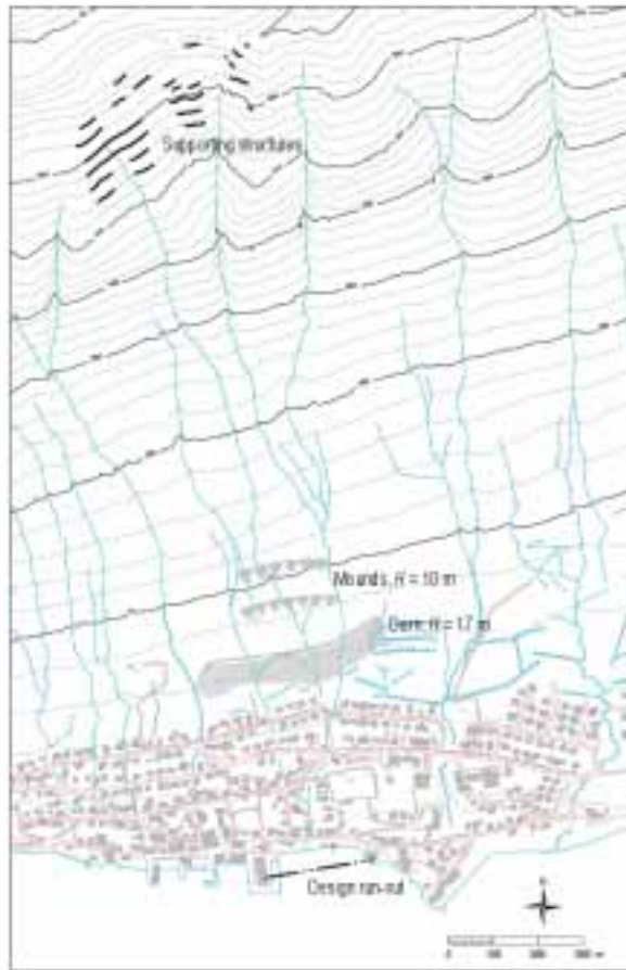
Figure D1: Protective measures in the Drangagil area at Neskaupstaður, eastern Iceland. The map shows the position of the supporting structures in the starting zone, two rows of braking mounds beneath the gully and a dam just above the uppermost houses. A closer map view, a photograph, and a vertical cross-section of the dam and mounds are shown in Figures 15.7, 15.8 and 15.9 in Section 15. Hazard zoning before and after the construction of the protection measures is shown in Figure G3.
