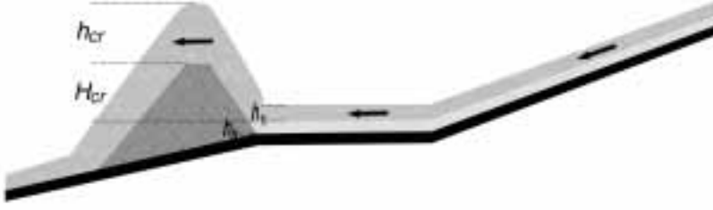
Figure 5.4: A schematic figure of supercritical overflow showing the critical dam height H_{cr} and the critical flow depth h_{cr} .
