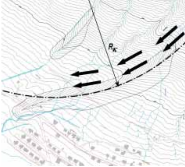
Figure 6.3: The deflection of an avalanche alongside the 700 m long, curved deflecting dam below Ytra-Strengsgil at Siglufjörður, northern Iceland. A circle with a radius of curvature R_k \approx 700 m has been fitted to the curved dam axis.
