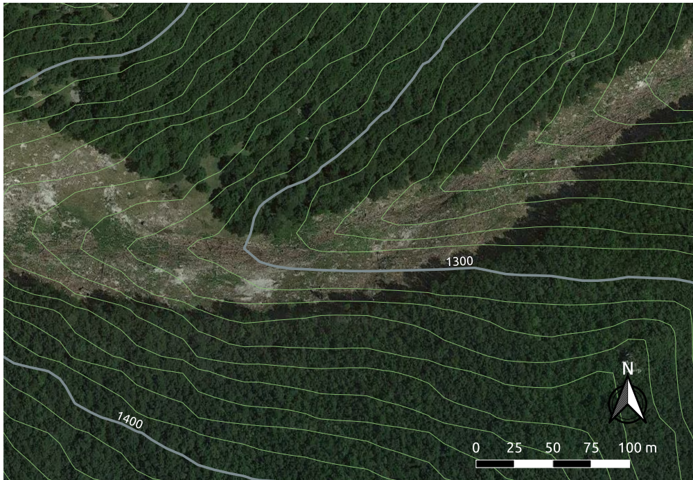
Figure 3 Detail from satellite image Fig. 3 in [1] around the left bend at 1300 m a.s.l. after the 2017 avalanche event. The trimline is at the transition from light foliage to dark green shadows. Equidistance of isolines 10 m
