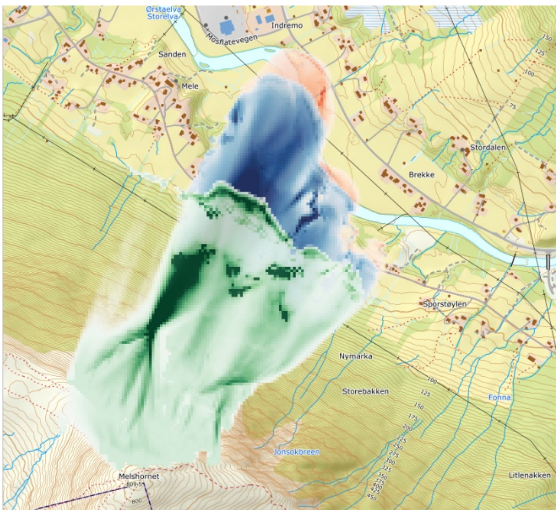
Figure 10. Comparison of simulations of an avalanche from the Melshorn, municipality of Volda. Green area is reached by the avalanche assuming the forest cannot be destroyed. The red area shows the run-out if the braking effect of the forest is ignored. The blue area results if the trees are destroyed once their bending strength is exceeded by the avalanche [NaturAct].
