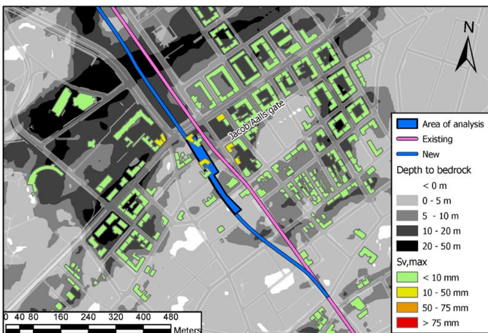
Figure 6 Result of impact classes only showing buildings that are not founded to/on bedrock, long-term scenario assuming permanent pore pressure reduction a) top: scenario A ( \Delta u_F = 100 kPa), b) bottom: scenario B ( \Delta u_F = 50 kPa).
