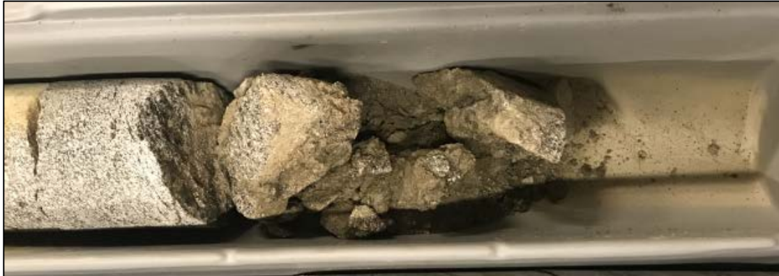
Figure 7. Zone with clay and crushed rock registered at 33.6-33.72 m. Subsequent to the crushed zone, 0.78 m with core loss is registered.
