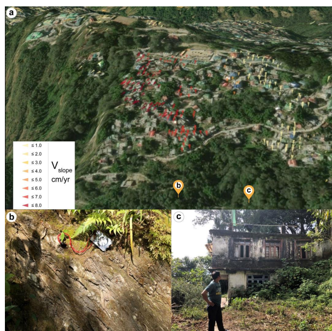
Figure 4. The InSAR observation and field investigation of Tathangchen landslide. (a) The Tathangchen sloping area in Gangtok, where the slope is moving at around 8–10 cm/yr. The mean velocities represent the projection of the vertical velocity field in the slope direction. (b) The rock outcrop shows highly weathered and foliated phyllitic rocks at the surface in Tathangchen. (c) Abandoned house due to settlements in the ground caused by creep at the Tathangchen area at an elevation of about 1638 m.
