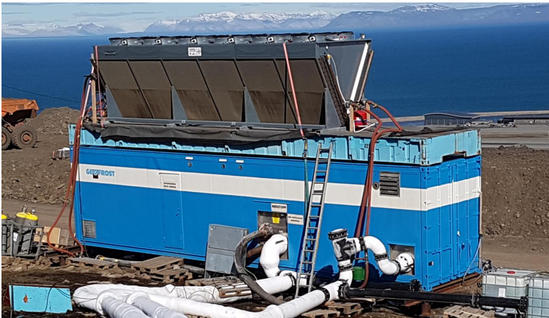
Figure 24: Freezing container and equipment for brine freezing. (Image courtesy of Anne-Lise Berggren, Geofrost AS).
