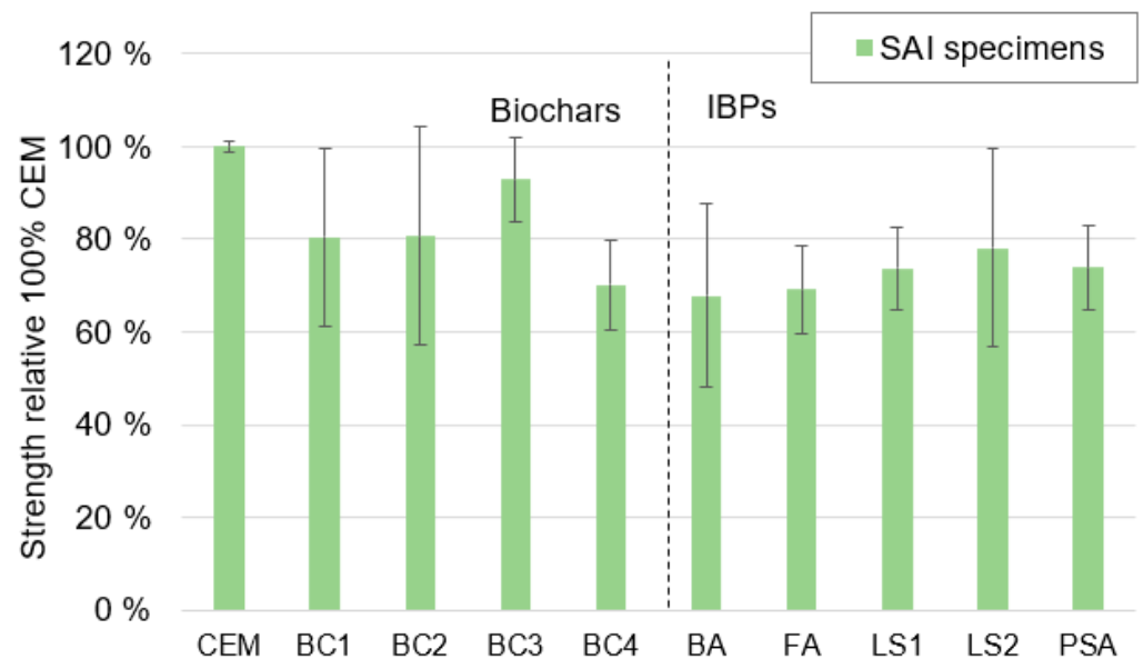
Figure 6. Results of the strength activity index (SAI) for 100% CEM and mixtures where 20% of the CEM was replaced with biochar or IBPs. Error bars show coefficients of variation.
