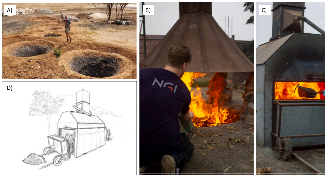
Fig. 1. a) Flame curtain “ Kon Tiki ” soil pit kilns in Zambia used to produce 100 t of biochar for a macadamia plantation, b) the soil pit kiln used for emissions testing in this study, c) el Horno , and d) schematic of el Horno .
