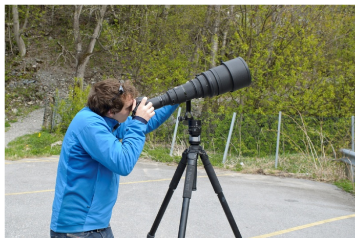
Figure 4. Manual Pano-Gimbal head with 400 mm and 2× teleconverter on D7000: effective focal length of 1,200 mm.
