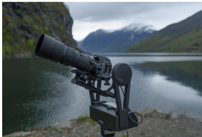
Figure 2. Giagapan Epic Pro set up with D7000 and 300 mm f4. Note that the no-parallax point (NPP) is behind the sensor plane.
