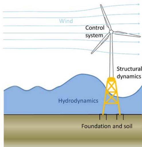
Figure 5 Loads and reaction included in integrated analyses.
