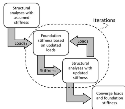
Figure 9 Iteration flow in computation of foundation stiffness
