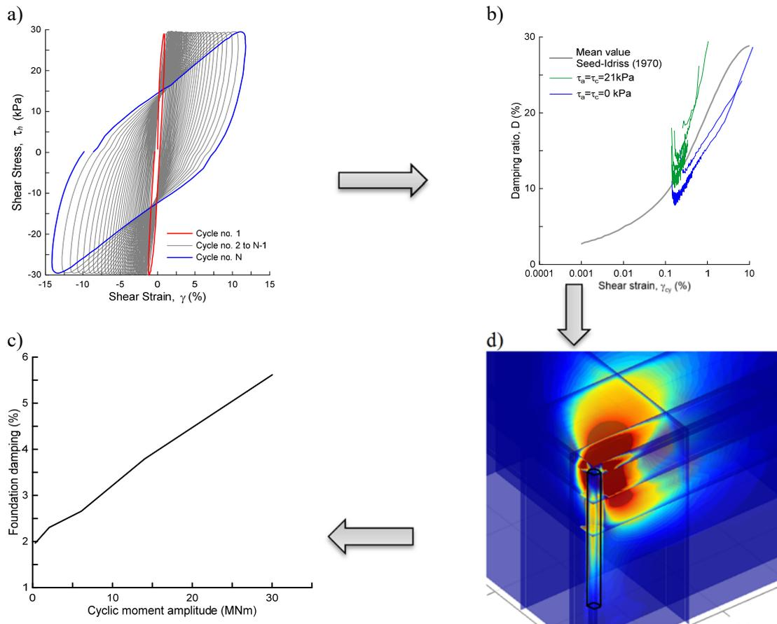
Figure 11 Computation of foundation damping. A) Laboratory sample testing, b) Extraction of damping for the soil element, c) Integration of the damping in soil volume d) Foundation damping as function of cyclic moment amplitude.
