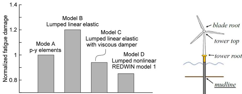
Figure 13 Foundation model influence on fatigue damage at tower root after [30].
