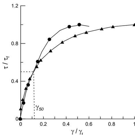
Figure 8 Stress-strain curves from two DSS tests on over consolidated North-sea clay
