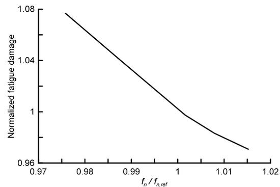
Figure 4 Effect of change in natural frequency on the accumulated fatigue damage (adapted from [5]).
