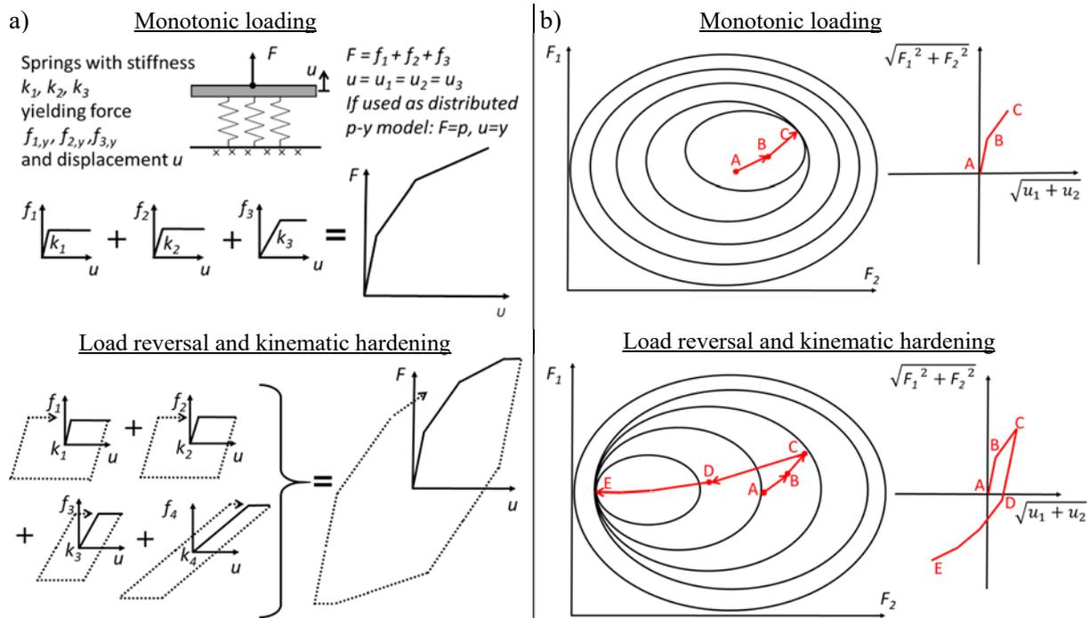
Figure 10 Illustration of the multi-surface plasticity concept a) 1D- parallel coupled principle, b) 2D-multi-surface translation in load space
