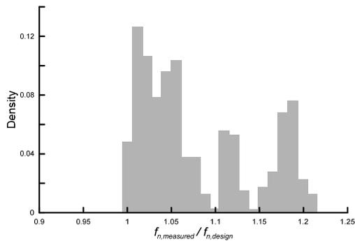
Figure 3 Measured natural frequencies versus frequency predicted in design for more 400 OWT (after [4]).
