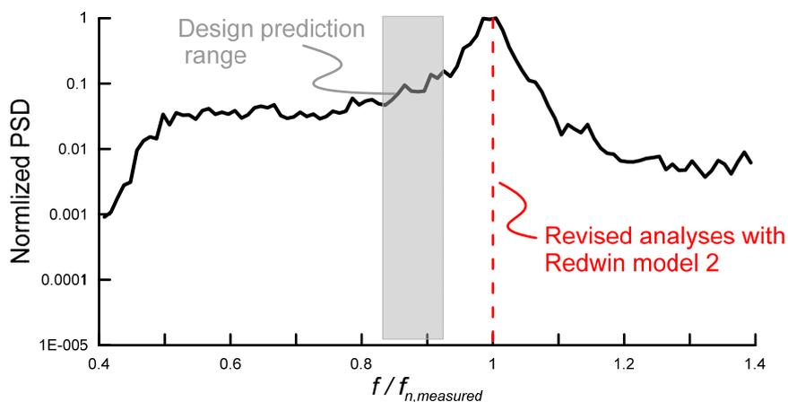
Figure 14 Peak spectral density from measurements showing natural frequency  $f_n$  of the first mode compared with original design natural frequency and natural frequency for analyses with Redwin model 2.
