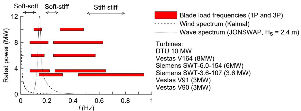
Figure 1 Load frequencies from wind, waves and blade rotation for some selected turbines (after Bak et al., 2013; Arany et al., 2016).
