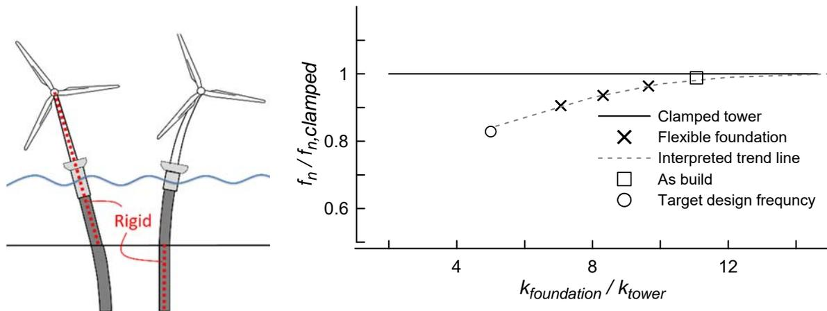
Figure 2 Dependence of OWT natural frequency on foundation stiffness a) Fully clamped foundation and fully rigid tower above mudline, b) OWT natural frequency as function foundation and tower stiffness ratio.
