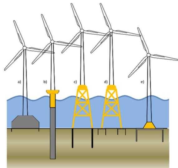
Figure 6 Foundation type considered in REDWIN project (OWTs not in scale).
