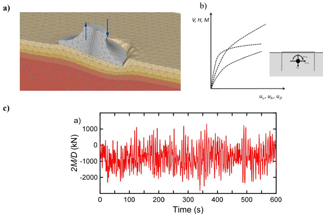
**Figure 12 Demonstration of model response. a) FEA of foundation with site specific data, b) Uniaxial load response as input to model, c) Macro-element response - Moment and rotation through a 10 min time history.**
