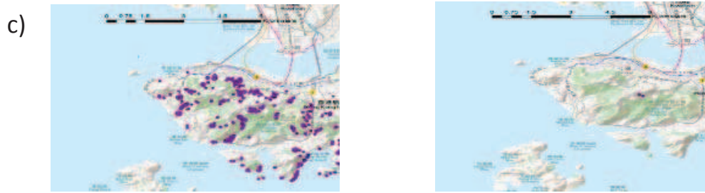
Figure 1. Landslide maps under storms of (a) 85% PMP; (b) 65% PMP; (c) 44% PMP; (d) 29% PMP.
