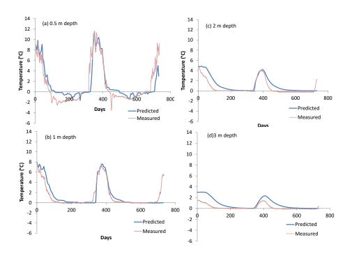
Figure 12: Comparison between measured and predicted variation of temperature at 4 different depths in BH6. Horizontal axis show the number of days from the initial date (12 Aug 2012).
