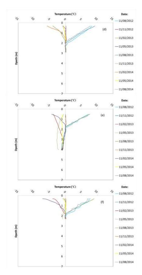
Figure 9: Variation of soil temperature at (a, d) BH4, (b, e) BH3 and (c, f) BH2 with (a, b, c) Time (the curves decrease in variation range with increasing depth) and (d, e, f) Depth.
