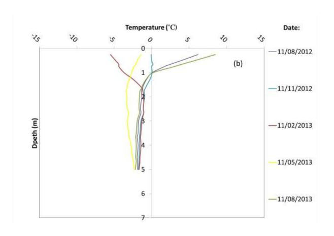
Figure 10: Variation of soil temperature at BH1 with (a) Time (the curves decrease in variation range with increasing depth) and (b) Depth.
