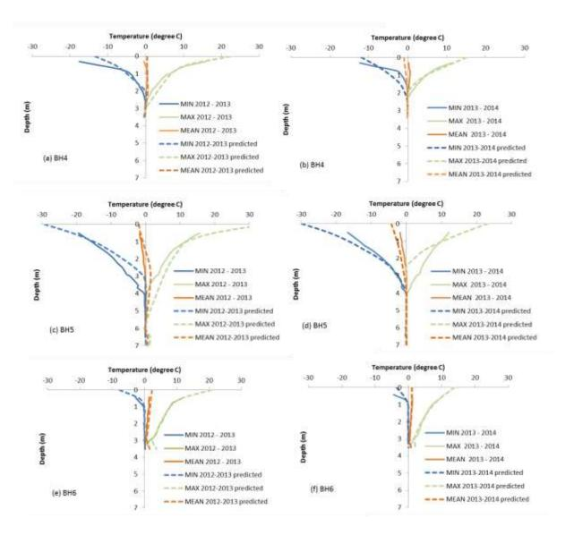
Figure 15: Measured and predicted trumpet curves for BH4, BH5 and BH6 from the 2D model
