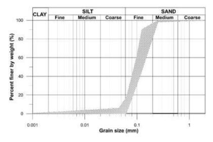
Figure 4: Grain size distribution (GSD) of soil samples from Pesyakov Island
