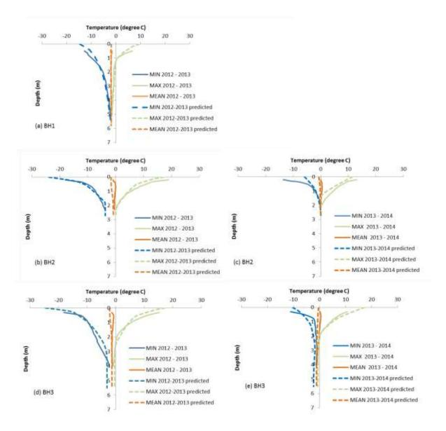
Figure 14: Measured and predicted trumpet curves for BH1, BH2 and BH3 from 1D models.
