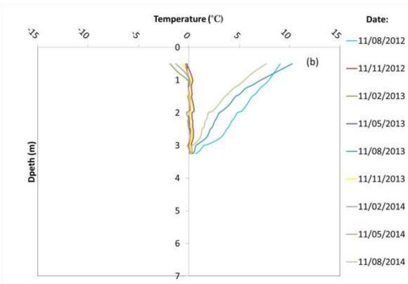
Figure 7: Variation of soil temperature at BH6 with (a) Time (the curves decrease in variation range with increasing depth) and (b) Depth.
