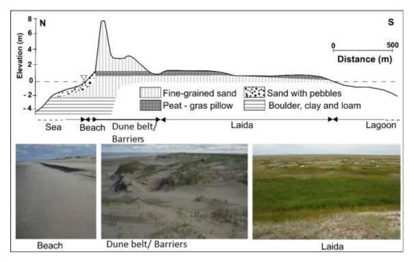
Figure 2: Schematic representation of a typical cross-section showing different morphological parts on Pesyakov Island (top figure), and pictures of the ground surface and topsoil at the beach, the dune belt and the laida (bottom sub-figures).
