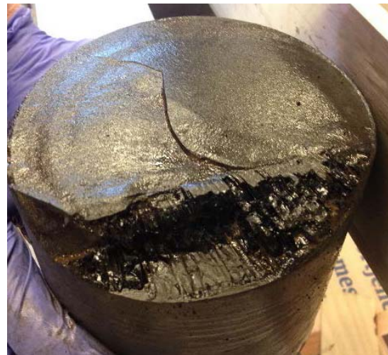
Figure 3 Index parameters and mineralogical composition of Draupne Shale (left table). Core photo of black Draupne Shale showing glossy shear surface with scattered striations and rough topography related to asperities (right).
