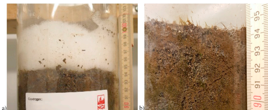
Fig. 2. a) The AFFF foam added to the soil columns. b) Foams bubbles visible in the soil after 24 h of water infiltration.
