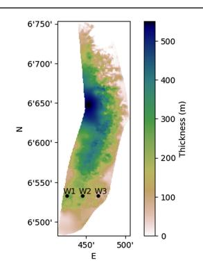
Fig. 1 Thickness map of the Skade formation with the 3 injection wells—W1, W2, and W3—marked
