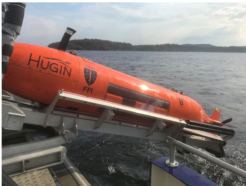
Figure 4. The HUGIN AUV equipped with a sensor payload including the HISAS system with capabilities for mapping the seabed and detecting gas seeps in the water column. This image was taken in Horten during the ACT4storage nearshore experiment.
