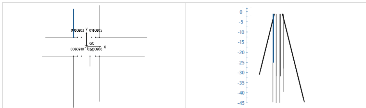
Figure 7. Illustration of pile group in GS PileGroup (Left: plan view, Right: depth profile view)
