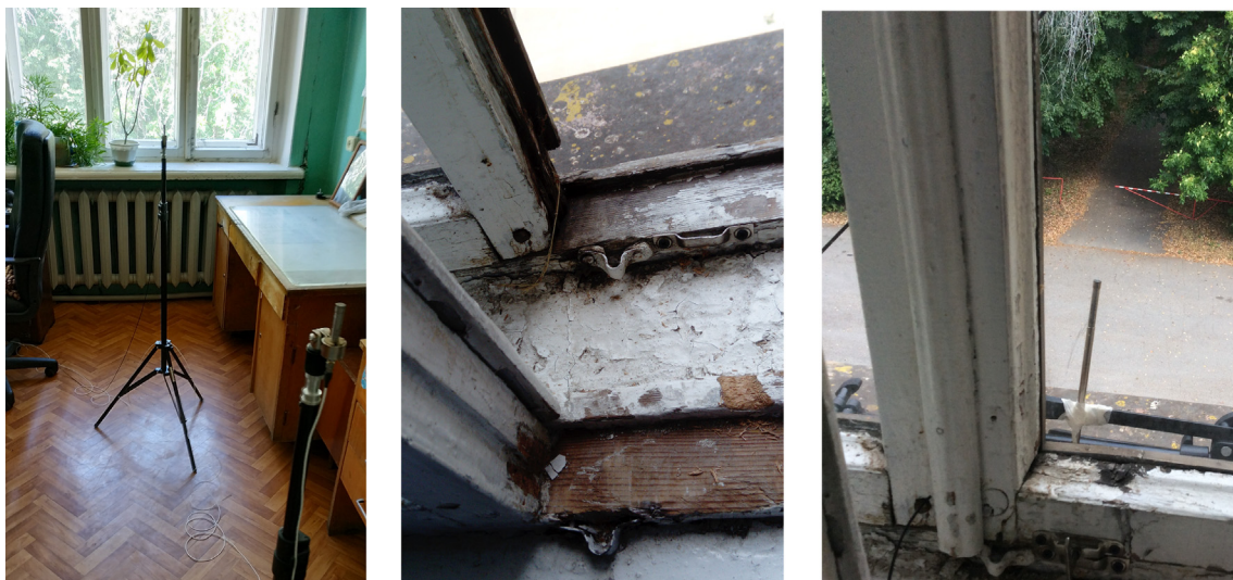
Fig. 4. Left: measurement room with microphone position no2 and no3 during flights 3-8 in 2019, middle: wooden double-pane unit windows, right: window with outdoor microphone in 2018.
